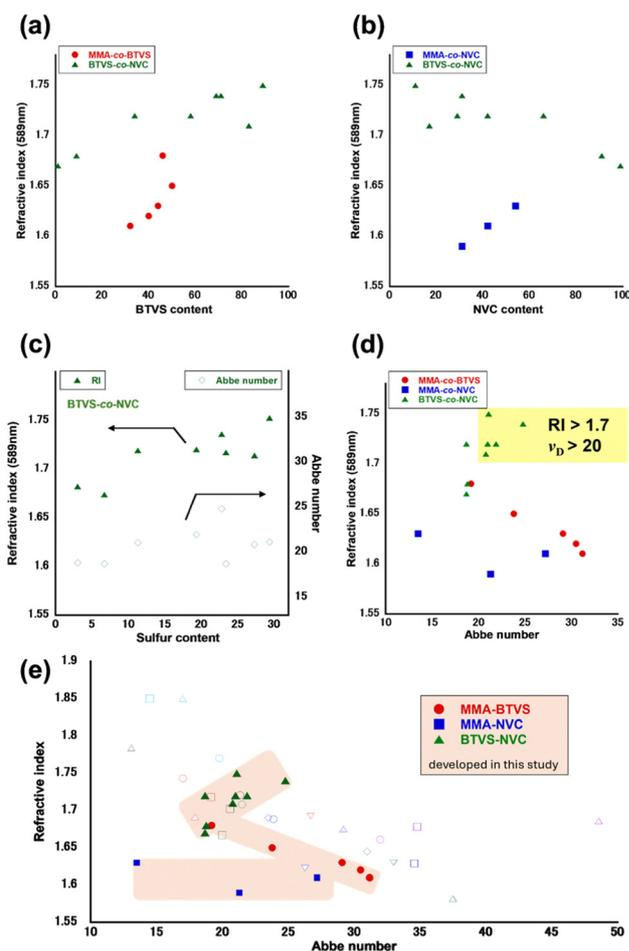
**Fig. 3** Correlations between (a) refractive index and BTVS content for BTVS-containing copolymers, (b) refractive index and NVC content for NVC-containing copolymers, (c) refractive index, Abbe number, and sulfur content for P(BTVS-*co*-NVC)s, and (d) refractive index and Abbe number for all copolymers. (e) Comparison between aromatic heterocycle-containing copolymers developed in this work and previously reported polymers (see Table S11 for detailed sample information).
