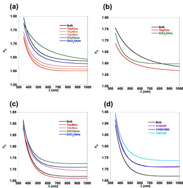
**Fig. 2** Wavelength-dependent refractive indices of the copolymer films, (a) P(MMA-co-BTVS)s, (b) P(MMA-co-NVC)s, and (c) P(BTVS-co-NVC)s prepared at a constant feed ratio (100/100) in different DESs, and (d) P(BTVS-co-NVC)s prepared at different feed ratios in ZnCl<sub>2</sub>/urea.
