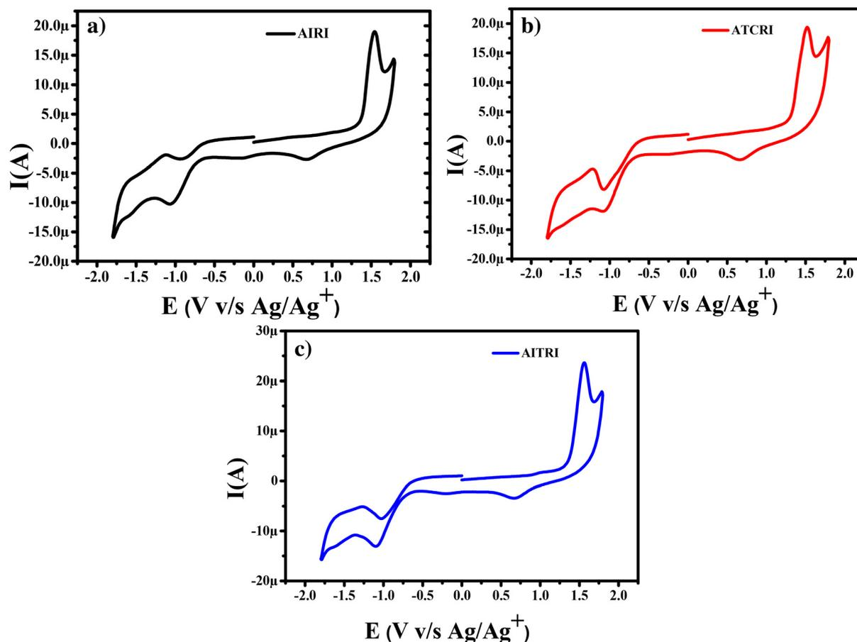
Fig. 4 Oxidation–reduction curves of the polymers, (a) AIRI (black line), (b) AICRI (red line) and (c) AITRI (blue line), obtained by cyclic voltammetry at  $50 \text{ mV s}^{-1}$  in dry acetonitrile–chloroform (7 : 3) using TBAPF<sub>6</sub> as a supporting electrolyte;  $E_{\text{Fc}/\text{Fc}^+}^{\text{onset}} = 0.38 \text{ V}$ .
