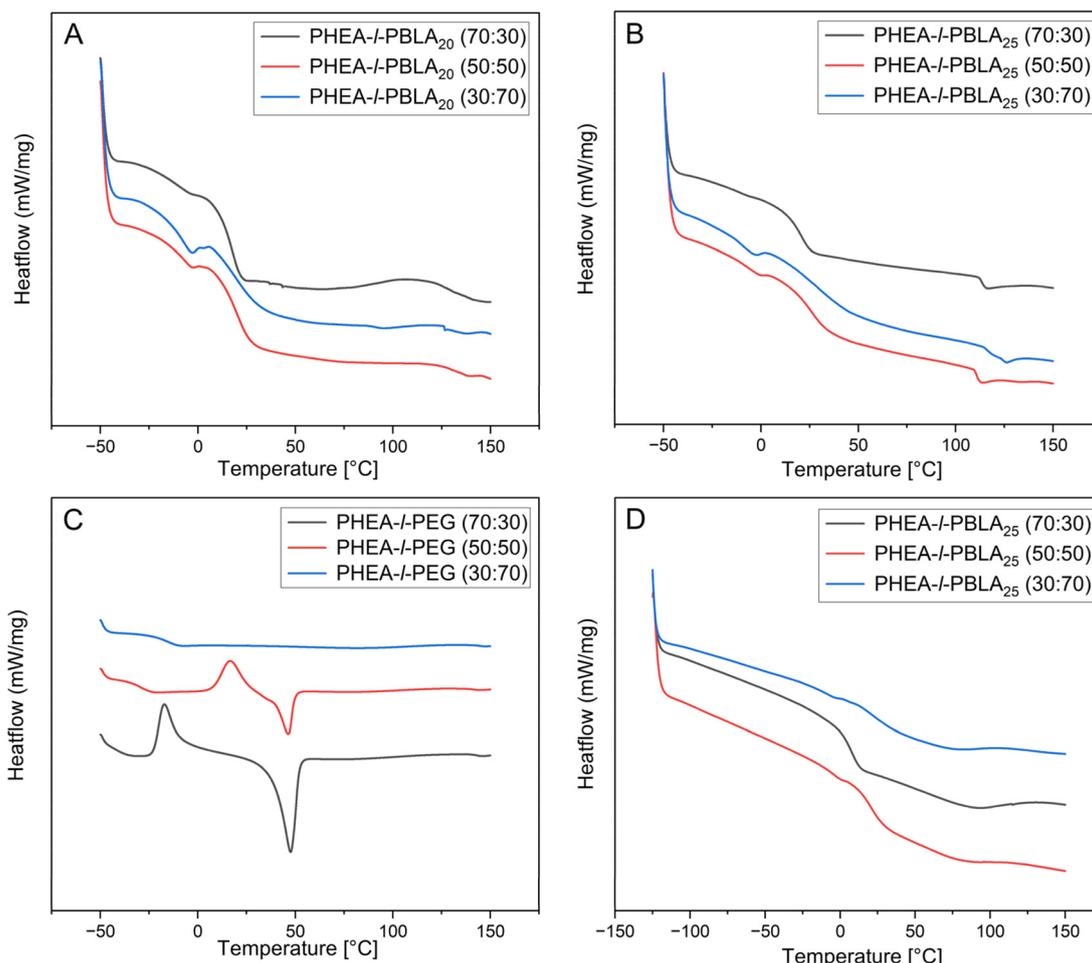
**Fig. 5** DSC thermograms (exothermic up) of PHEA-*l*-(PBLA-*b*-PEG-*b*-PBLA) and PHEA-*l*-PEG conetworks. (A) PHEA-*l*-PEG. (B) PHEA-*l*-PBLA<sub>25</sub>. (C) PHEA-*l*-PBLA<sub>20</sub> measured from  $-50$  °C to  $150$  °C. (D) PHEA-*l*-PBLA<sub>25</sub> measured from  $-125$  °C to  $150$  °C. All thermograms show the second heating cycle.
