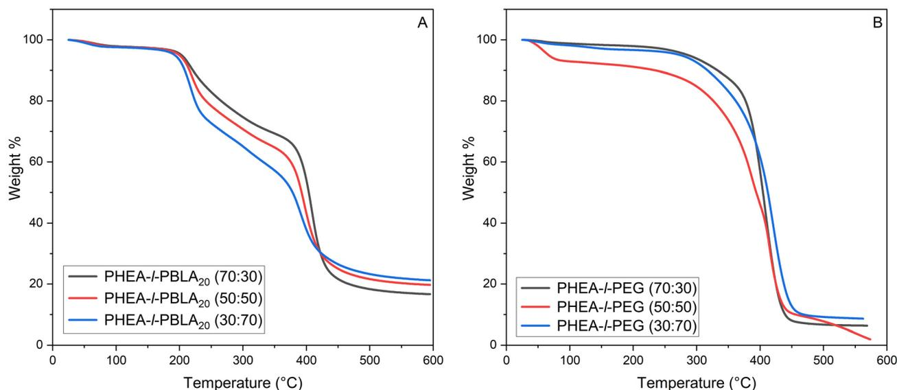
Fig. 6 TGA thermograms of (A) PHEA-*l*-(PBLA-*b*-PEG-*b*-PBLA) and (B) PHEA-*l*-PEG conetworks.
