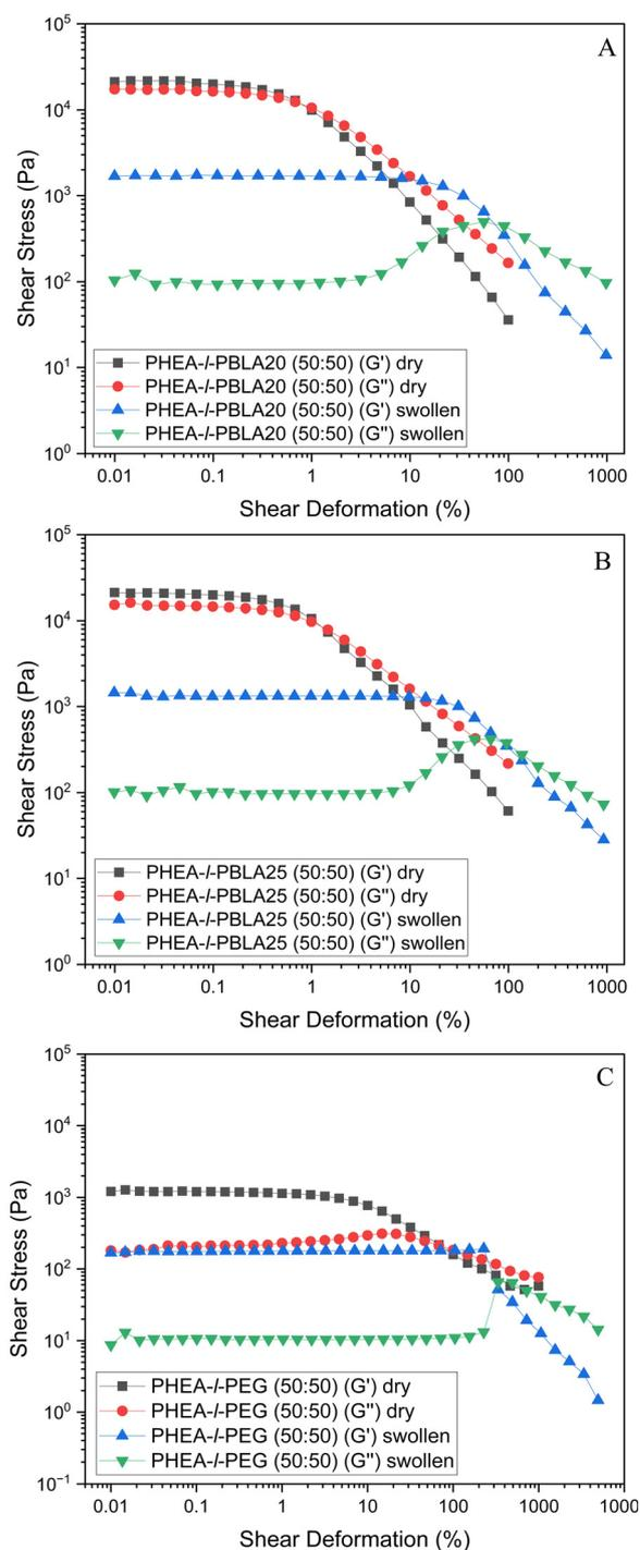
**Fig. 9** Rheology data of dry and water-swollen PHEA-*l*-(PBLA-*b*-PEG-*b*-PBLA) and PHEA-*l*-PEG conetworks with a 50:50 wt% composition. (A) PHEA-*l*-PBLA<sub>20</sub>, (B) PHEA-*l*-PBLA<sub>25</sub>, and (C) PHEA-*l*-PEG.
