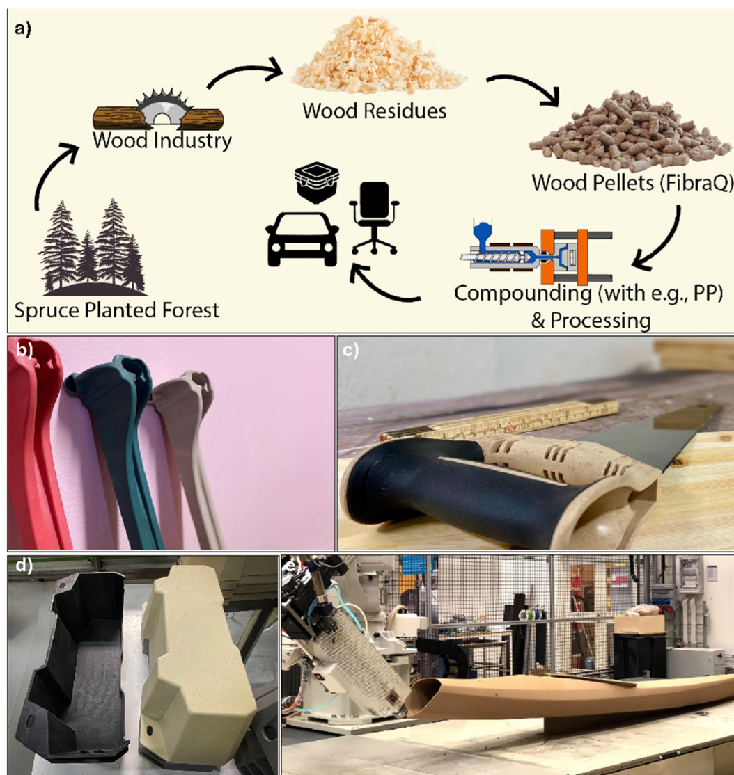
Fig. 1 Production and applications of wood fiber pellets in biocomposites: (a) schematic representation of the circular value chain: sustainably managed spruce forests provide processing residues that are densified and pelletized to yield standardized wood fiber pellets, which are subsequently screened to remove fines, and compounded into biocomposite materials for commercial product manufacturing. (b–d) Examples of injection-molded products produced from wood fiber composite formulations; (c) component part illustrating a rigid polypropylene/wood fiber structure overmolded with a thermoplastic elastomer (TPE). (e) Large-format additive manufacturing demonstrated by the fabrication of a full-size, 3D-printed (FDM) kayak from wood fiber-reinforced recycled plastics, developed in partnership with RISE Research Institutes of Sweden and Melker of Sweden using FibrAQ. 26
