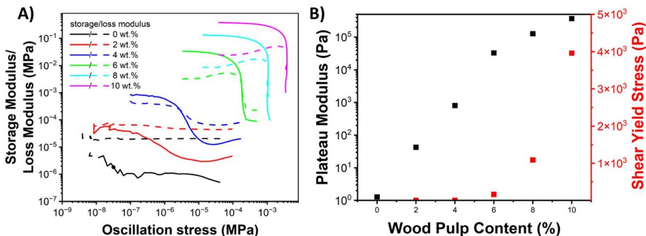
Fig. 2 Rheological studies on the epoxy composites including a stress sweep and its corresponding (A) storage ( $G'$ ) and loss modulus ( $G''$ ) at varying oscillation stress and (B) plateau modulus and shear yield stress at varying wood pulp content.
