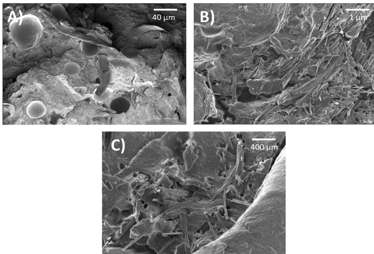
**Fig. 5** SEM images of the fracture surface of printed wood-pulp and nanoclay (Garamite) filled resin featuring (A) voids due to printing and the presence of wood pulp, and (B/C) fiber and nanoclay pull out.
