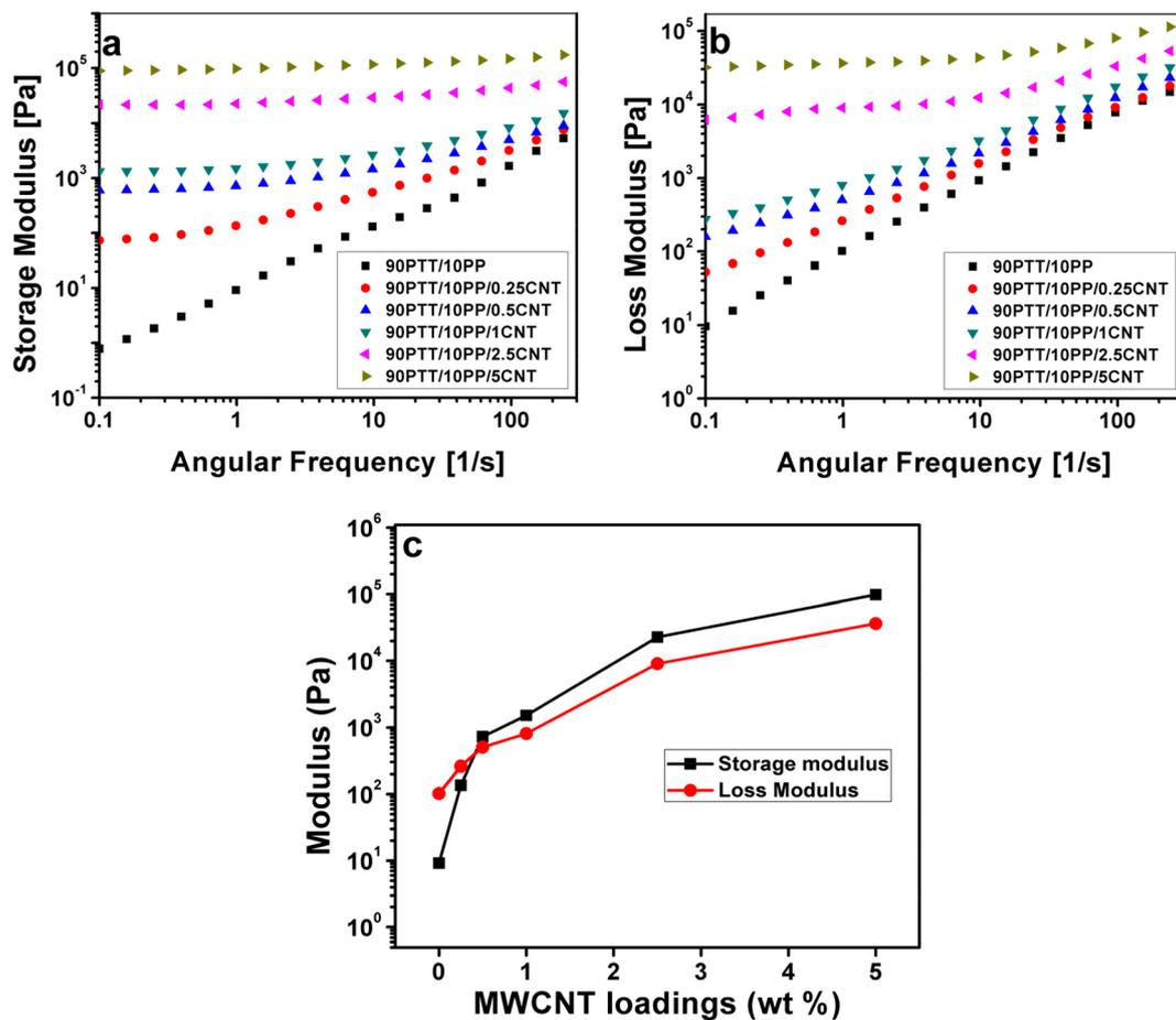
Fig. 11 Variation of (a)  $E'$ , (b)  $E''$  and (c) comparison between  $E'$  and  $E''$  as a function of MWCNT loading at 0.1 rad s<sup>-1</sup>.
