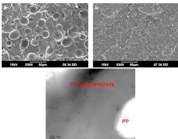
**Fig. 2** Scanning electron microscopy images of (a) the 90PTT/10PP blend, (b) 90PTT/10PP/1MWCNTs and (c) TEM image of 90PTT/10PP/1MWCNTs, showing preferential localization of CNTs within the PTT-rich phase and evidence of interfacial confinement.
