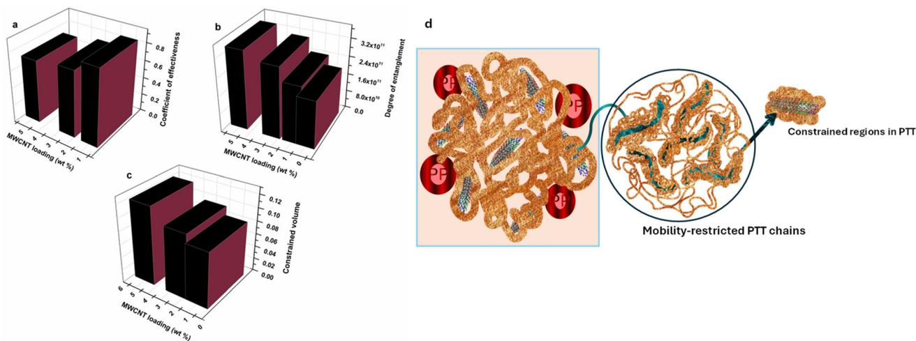
**Fig. 10** Variation in the (a) effectiveness of dispersion,  $E_f$ , (b) degree of entanglement,  $\phi$ , and (c) volume of the constrained region in the PTT matrix with MWCNT loading in the 90PTT/10PP blend; (d) schematic representation of the development of a constrained region in 90PTT/10PP/MWCNT composites. It represents how CNT preferential localization in the PTT phase restricts nearby chain mobility and produces a confined nanophase.
