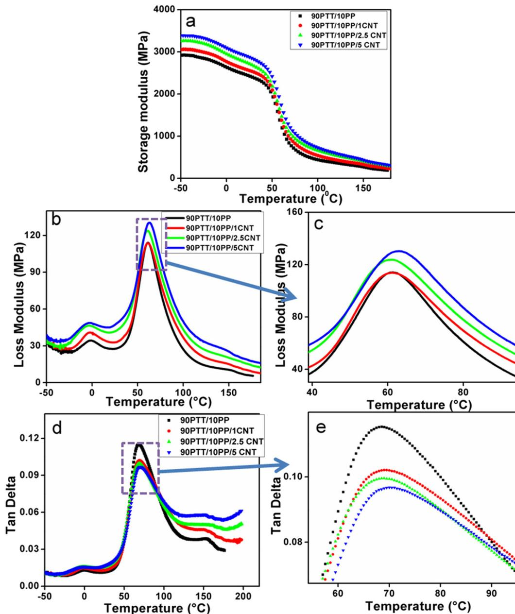
Fig. 9 Plot of DMA analysis of 90PTT/10PP blends with different MWCNT loadings: (a)  $E'$ , (b)  $E''$ , (c) magnified image of  $E''$  versus temperature for the PTT phase, (d)  $\tan \delta$  versus temperature, and (e) magnified portion from the graph of  $\tan \delta$  versus temperature peak of the PTT phase.
