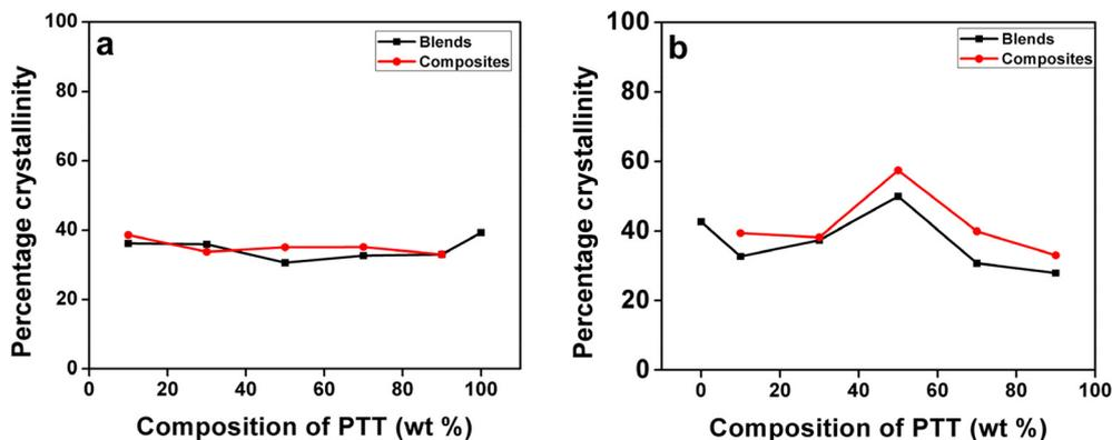
Fig. 7 Crystallinity of (a) PTT and (b) PP in blends and composites (values calculated using standard enthalpy from DSC data).
