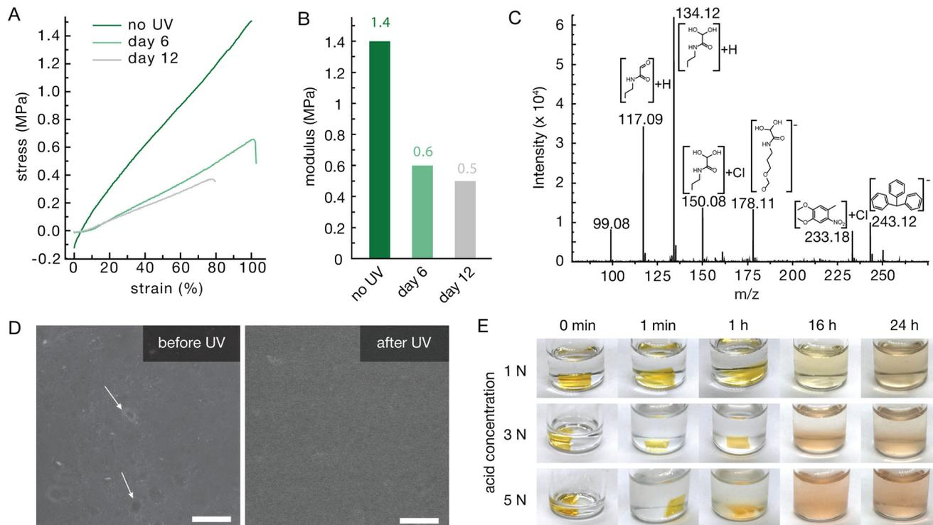
**Fig. 3** (A) Stress strain curve showing pull to break tests before UV exposure, 6 days after UV exposure and 12 days after UV exposure (B) and the respective Young's moduli. (C) DART-MS of the 5k 10 mol percent crosslinked PETg after acid exposure. (D) SEM of the 5k 10 mole percent cross-linked PETg before and after UV exposure. (E) Photographs at timepoints during exposure to varied concentrations of hydrochloric acid.
