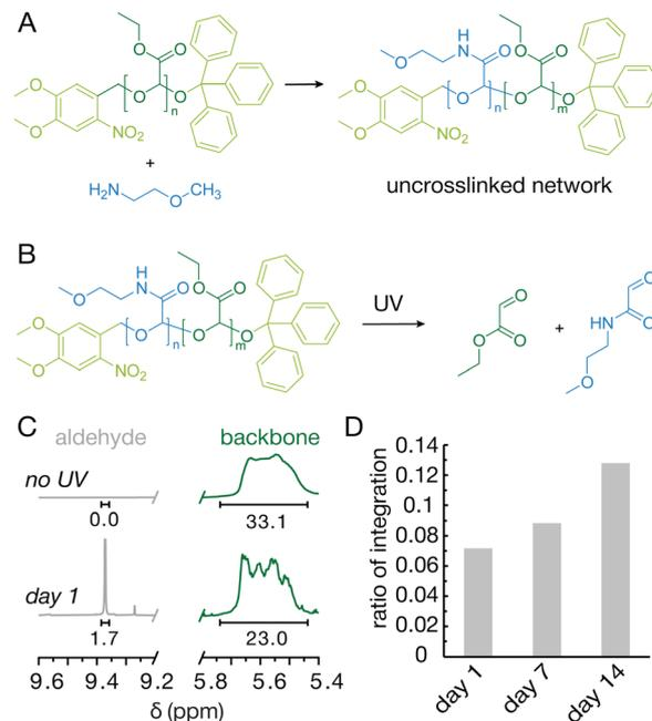
**Fig. 4** (A) Reaction scheme of PETg with monoamine to create a soluble sample for NMR analysis. (B) Depolymerization of PETg with appended monoamine on exposure to UV light. (C) Zooms of NMR spectra showing the appearance of an aldehyde peak. (D) Ratio of integration of the aldehyde peak to the backbone peak after UV exposure on day 1, 7 and 14.
