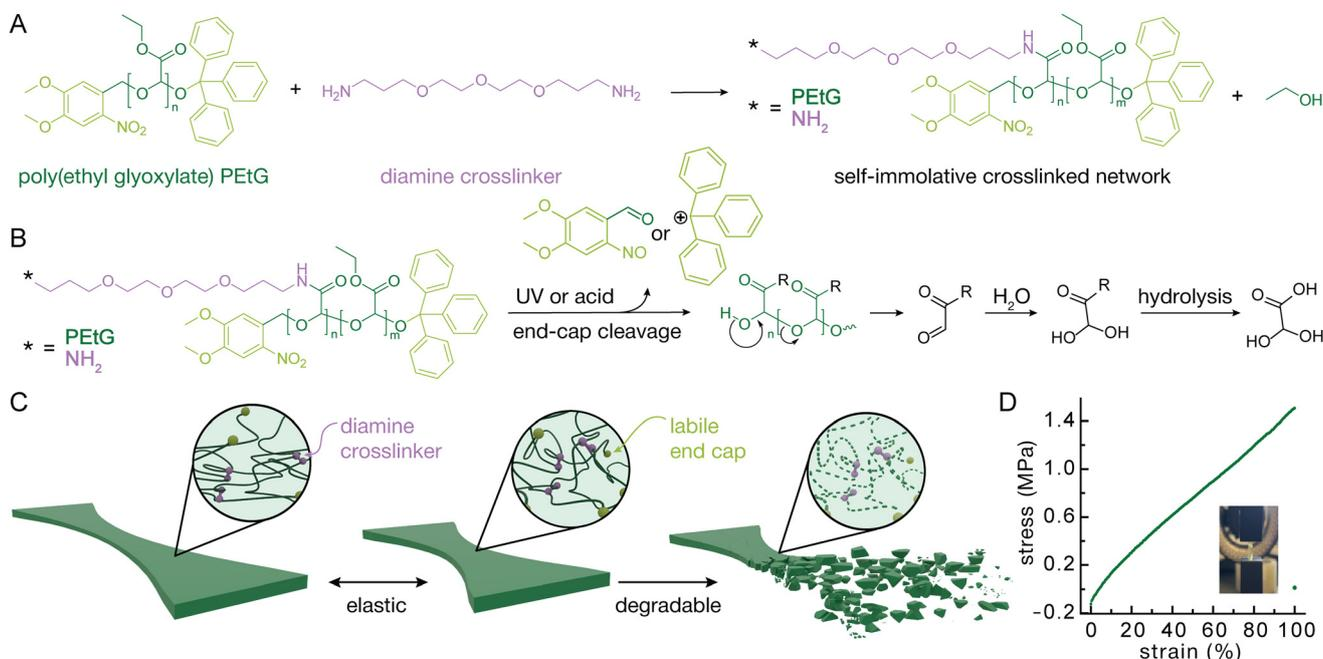
**Fig. 1** (A) Crosslinking of PEtG with a diamine to create crosslinked polymer network. (B) Depolymerization triggered by UV light or acid and subsequent hydrolysis of the product. (C) Scheme to show the stretching and degradation of the bulk material. (D) Representative example stress strain curve for the crosslinked material.
