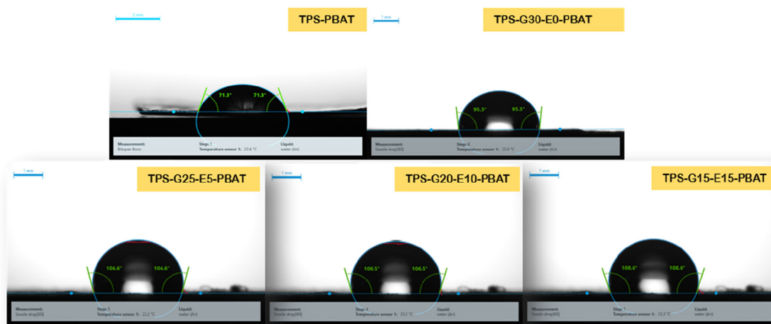
Fig. 4 Contact angle of the composite thin films.
