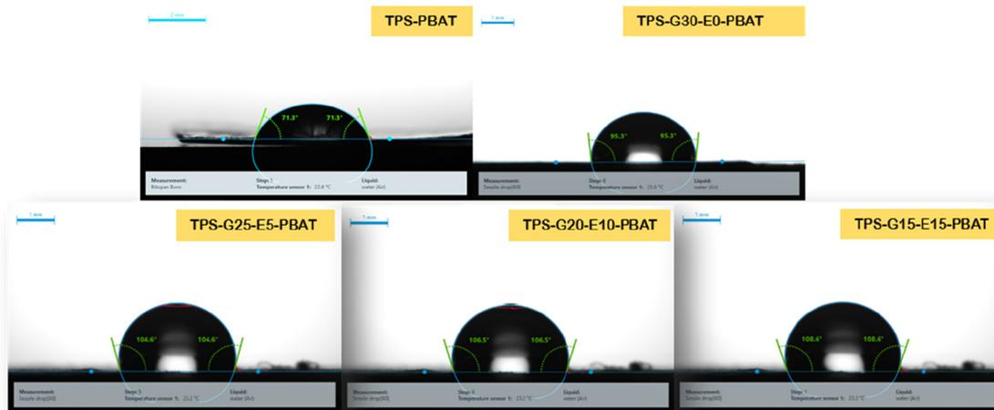
Fig. 4 Contact angle of the composite thin films.
