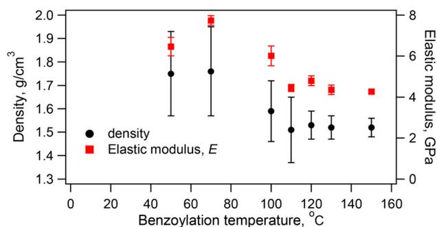
Fig. 4 Plot of the densities and elastic moduli,  $E_b$ , of the compacts of benzyated composites against benzylation temperatures. The standard errors obtained from three to four measurements were represented by error bars.
