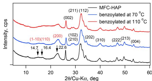
**Fig. 3** XRD patterns of the parent MFC–HAP composite and the benzoylated MFC–HAP composites. The indices of the diffraction peaks of HAP and those of cellulose I <sub>$\beta$</sub>  are shown in black and red, respectively.
