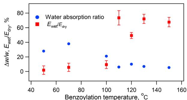
**Fig. 7** Plot of the water absorption ratios,  $\Delta w/w$ , and the ratios of the elastic moduli,  $E_{\text{wet}}/E_{\text{dry}}$ , of the benzoylated composite compacts against benzoylation temperatures. The standard errors obtained from three to four measurements were represented by error bars.
