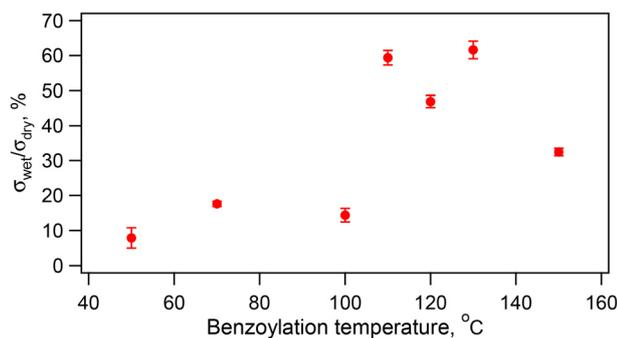
**Fig. 8** Plot of the ratios of bending strengths of the wet compacts to those of the dry compacts ( $\sigma_{\text{wet}}/\sigma_{\text{dry}}$ ) against benzoylation temperatures. The standard errors obtained from three to four measurements were represented by error bars.
