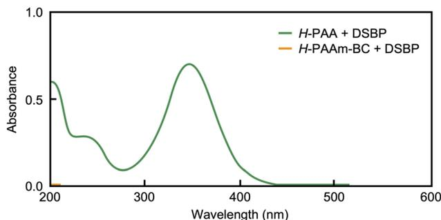
Fig. 3 UV spectra of the DSBP-PAA and DSBP-PAAm-BC mixtures. DSBP/AAm = DSBP/AA = 0.5.  $[AA]_0 = [AAm-BC]_0 = 3.57 \times 10^{-3}$  mol L<sup>-1</sup>.
