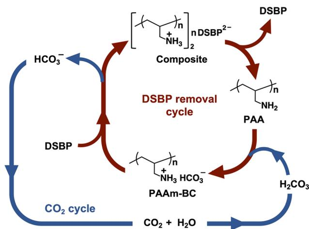
Fig. 1 Schematic illustration of DSBP removal by PAAm-BC in a closed-loop CO<sub>2</sub> cycle.
