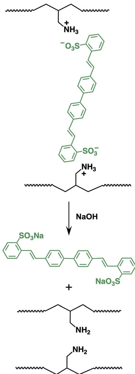
Fig. 12 Release of DSBP from the polymer composites under basic conditions.
