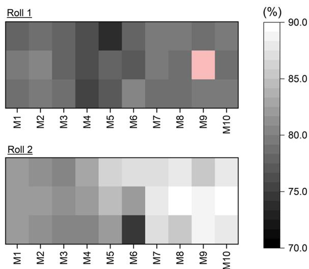
**Fig. 2** Low resolution maps showing the variation in crystallinity along and between two commercial HDPE rolls supplied by Goodfellows. The pink sample in roll 1 signifies a sample that was lost before analysis.
