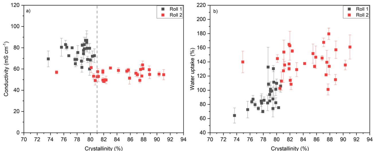
**Fig. 6** (a) Scatter plot showing the relationship between crystallinity and conductivity where the black squares indicate values from roll 1 and the red squares shows values obtained from roll 2. The dashed line at 82% marks the threshold at which crystallinity appears to no longer impact conductivity. (b) Scatter plot showing the relationship between crystallinity and WU where the black squares indicate values from roll 1 and the red squares shows values obtained from roll 2.
