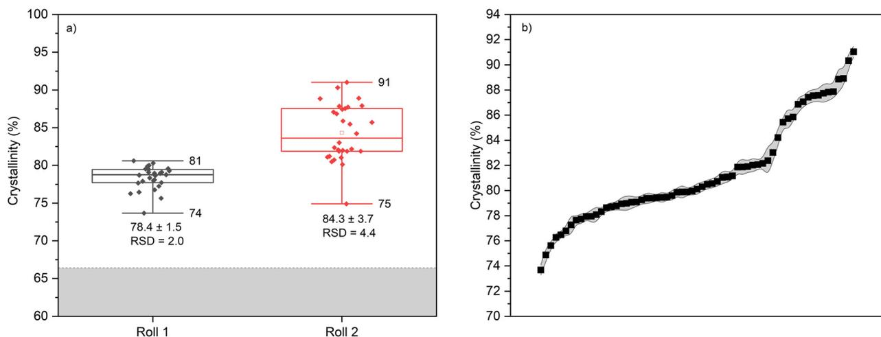
**Fig. 3** Box plot showing the measured variation in crystallinity between rolls 1 and 2. The area shaded grey shows the degree of crystallinities threshold for PE (defined high density  $> 0.944 \text{ g cm}^{-3}$ ). (b) The mean crystallinities of the samples (across all rolls) arranged in order of increasing crystallinity (left to right) with the sample standard deviations ( $n = 10$  repeat measurements on each sample) given as the grey zone.
