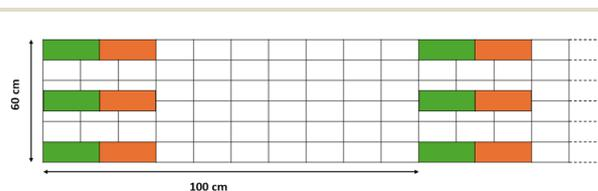
**Fig. 1** A cartoon depicting the sample locations within the 60 cm  $\times$  10 m commercial rolls. The green rectangles denote the areas used to calculate crystallinity (*via* density measurements), whilst the orange rectangles show the area used for the synthesis of the RG-AEMs. These samples were taken at every 1 m intervals along the roll.
