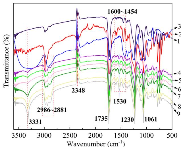
**Fig. 3** FTIR spectra of PVA/PPC-PU/PPC-X composites (1: PPC-X; 2: PPC-PU; 3: preplasticized PVA. 4–9:  $x\text{PVA}/y\text{PPC-PU}/z\text{PPC-X}$  (wt%) = 20/30/50, 30/10/60, 30/20/50, 30/30/40, 30/40/30, 40/30/30).
