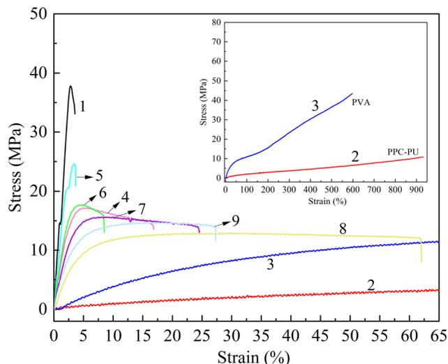
**Fig. 1** Tensile stress-strain curves of typical PVA/PPC-PU/PPC-X composites (1: PPC-X; 2: PPC-PU; 3: preplasticized PVA. 4–9:  $x\text{PVA}/y\text{PPC-PU}/z\text{PPC-X} = 20/30/50, 30/10/60, 30/20/50, 30/30/40, 30/40/30, 40/30/30$ ).
