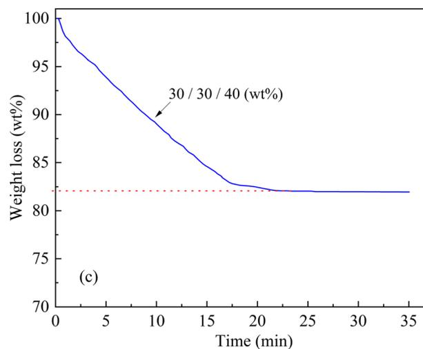
**Fig. 5** Thermogravimetric analysis of PVA/PPC-PU/PPC-X composites: (a) TGA; (b) DTG; (c) ITG (isothermal TGA) (1: PPC-X; 2: PPC-PU; 3–9: xPVA/yPPC-PU/zPPC-X (wt%) = 0/30/70, 20/30/50, 30/10/60, 30/20/50, 30/30/40, 30/40/30, 40/30/30. 10: preplasticized PVA).
