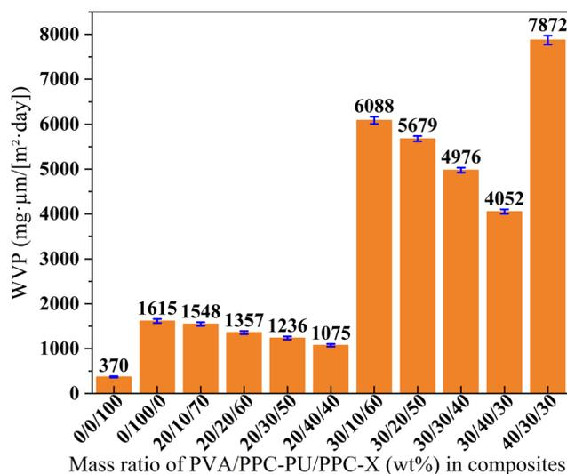
Fig. 10 Water vapor permeability coefficient of PVA/PPC-PU/PPC-X composite films (xPVA/yPPC-PU/zPPC-X, wt%).
