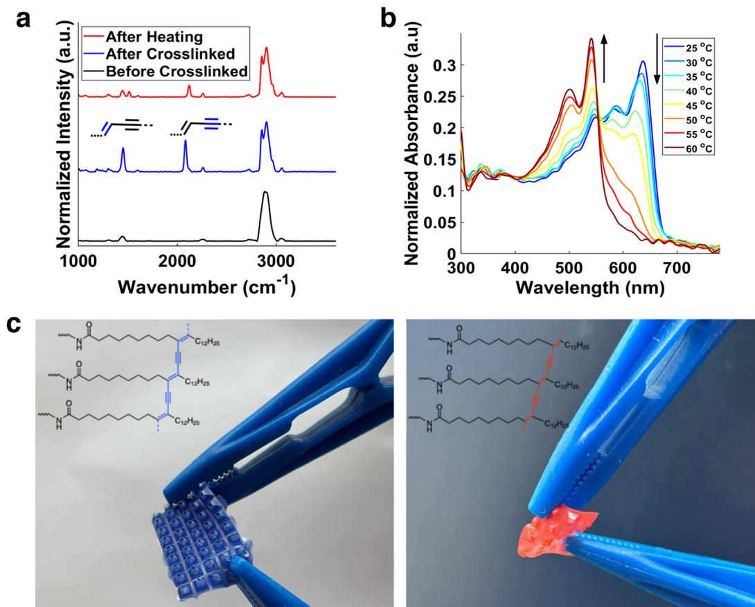
**Fig. 3** Photocrosslinking of the composite. (a) Raman spectroscopy analysis for SEBS-PDA composite before crosslinked (black), after crosslinked (blue), polymer after heating (red); (b) UV-vis spectra of SEBS-PDA-crosslinked composite films from 25–60 °C, and (c) SEBS-PDA photocrosslinked composite before (left) and after (right) heating to 60 °C.
