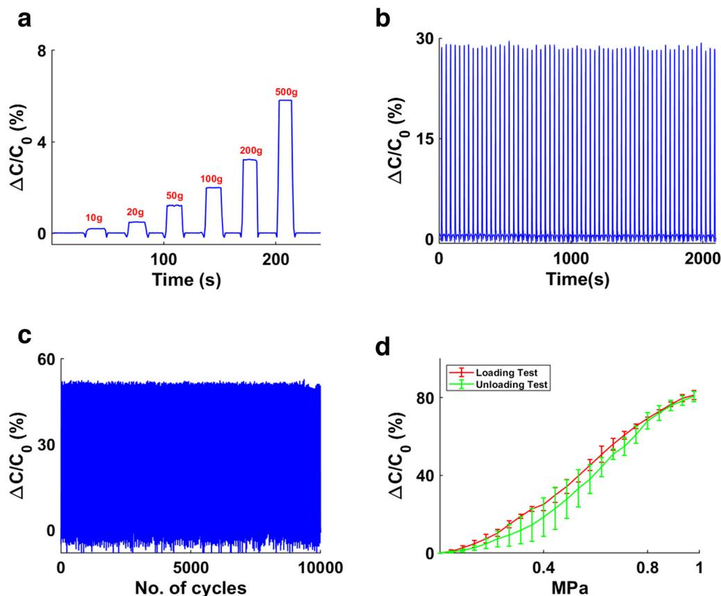
**Fig. 4** Pressure sensing characteristics of the SEBS–PDA blend sensor at room temperature. (a) Relative capacitances change under ascending pressure (b) cyclic loading at 55 N; (c) fatigue tests at 220 N for 10 000 cycles, and (d) hysteresis plot for loading and unloading (0–480 N).
