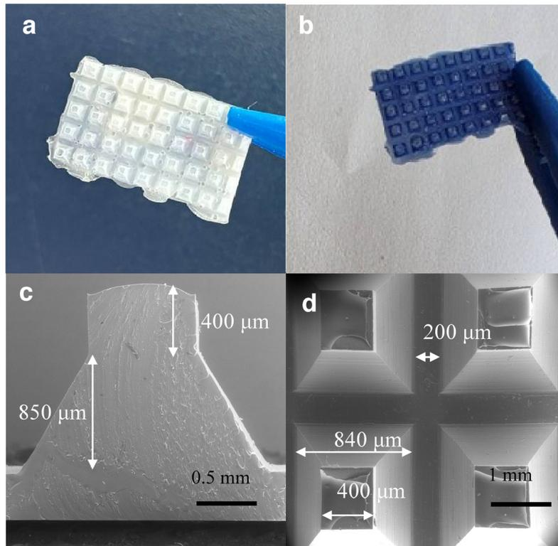
**Fig. 2** Patterning of the SEBS-PDA composite. Photography of MAP-patterned dielectric materials (a) before and (b) after irradiation with UV (254 nm); scanning electron microscopy (SEM) image of (c) lateral and (d) cross-section of the MAP structure. Scale bars are respectively 0.5 and 1 mm.
