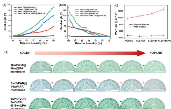
**Fig. 6** (a and b) Bend angles of the various bilayered membranes in humidification and dehumidification processes, (c) WVT rates of the various bilayer membranes without windows and with windows, and (d) optical images of the humidity-responsive behavior of the PA/PA membrane, PAN/PA membrane, and PVDF/FPU/PA membrane.
