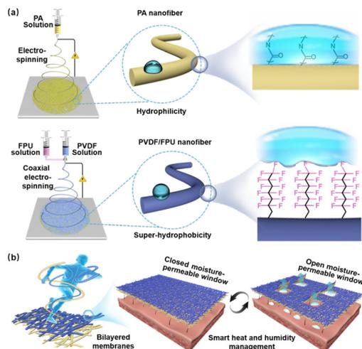
**Fig. 1** (a) Schematic illustration of the fabrication and structure of bilayered membranes. (b) Schematic demonstration of the smart heat-humidity management of bilayered membranes.
