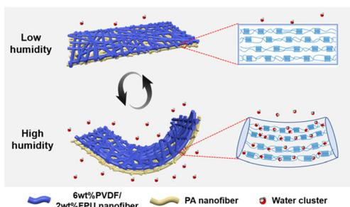
**Fig. 5** Schematic demonstration of humidity-responsive bilayered membranes.
