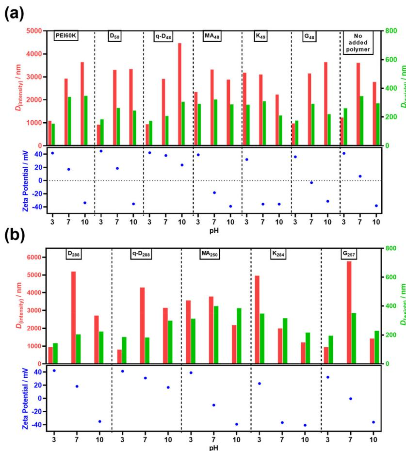
**Fig. 2** Zeta potential (blue dots), intensity-average diameter  $D_{\text{intensity}}$  (red columns) and weight-average diameter  $D_{\text{weight}}$  (green columns) of IOP dispersions with different added polymers at pH = 3, 7 and 10. The IOP concentration was 0.1% w/w based on the mass of the dispersion, and the added polymer concentration was 1% w/w based on the mass of the IOPs.
