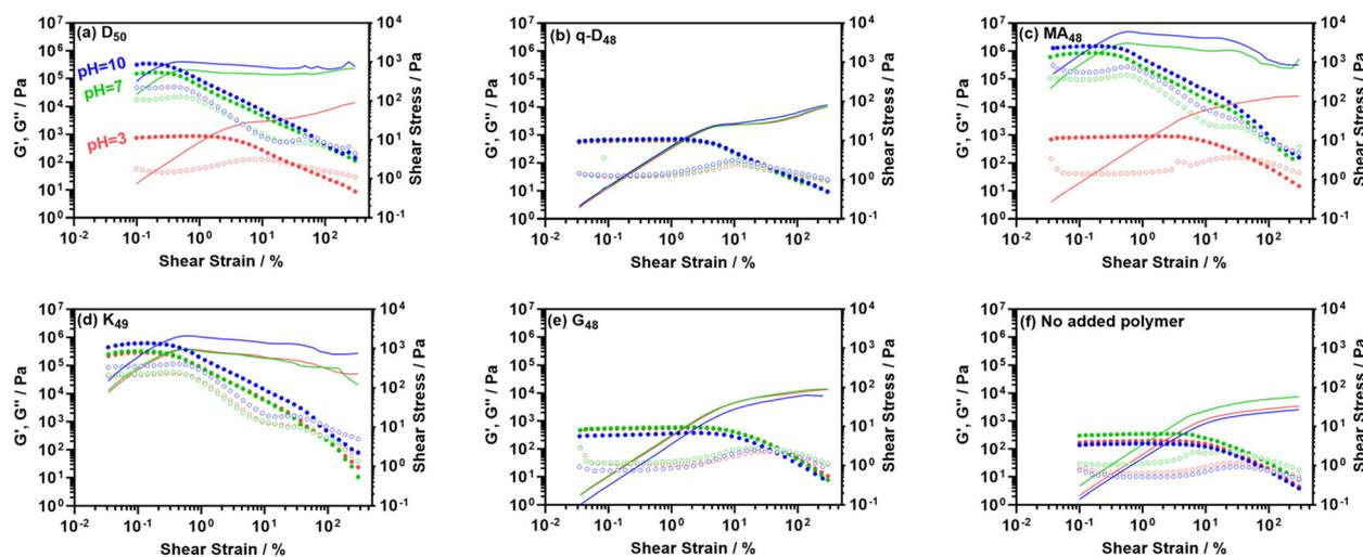
**Fig. 5** Storage modulus ( $G'$ , solid dots), loss modulus ( $G''$ , hollow dots) and shear stress (solid lines) as a function of shear strain for 50% w/w IOP suspensions with 0.5% w/w (a)  $D_{50}$ , (b)  $q-D_{48}$ , (c)  $MA_{48}$ , (d)  $K_{49}$ , (e)  $G_{48}$ , and (f) without added polymer at pH = 3 (red), pH = 7 (green) and pH = 10 (blue). The 0.5% w/w polymer additive concentration is based on IOP concentration.
