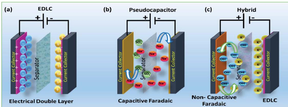
**Fig. 36** Charge storage mechanism of supercapacitors, (a) EDLCs, (b) pseudocapacitors and (c) hybrid supercapacitors.<sup>551</sup> Reproduced with permission from RSC.
