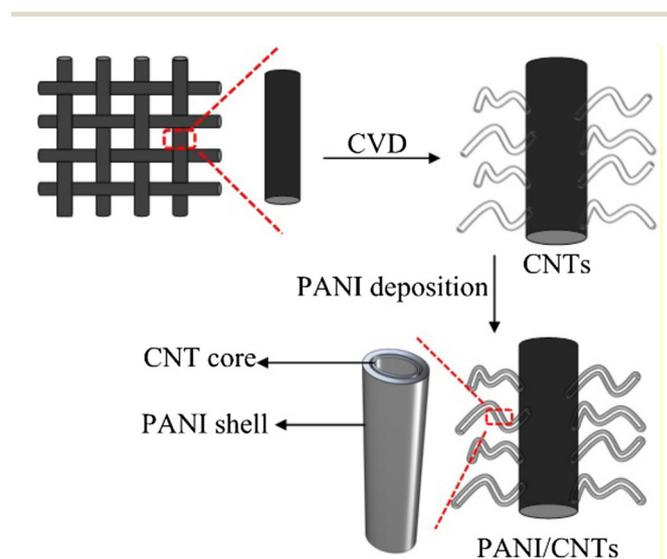
**Fig. 40** Illustrations of the fabrication process for PANI/CNTs on carbon cloth (CC).<sup>606</sup> Reproduced with permission from Springer.
