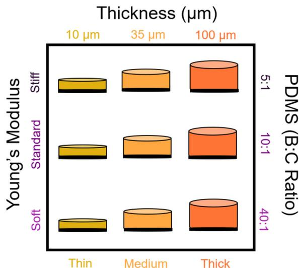
**Fig. 1** Schematic of the nine PDMS gels evaluated in this study. Throughout the results section, we will refer to a PDMS gel by their thickness and stiffness (bottom and left axes, respectively). The B : C ratio used to fabricate PDMS gels with different stiffnesses is noted on the right axis.
