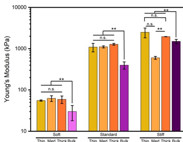
**Fig. 2** The Young's moduli of spin-coated PDMS gels as a function of their thickness was acquired using FFM AFM. Rheological measurements on “bulk” 5 mm thick gels are also provided.<sup>42</sup> The error bars denote standard deviation. Two asterisks (\*\*) denote that the values are significantly different at 0.01 level, whereas n.s. indicates that the samples are not statistically different.
