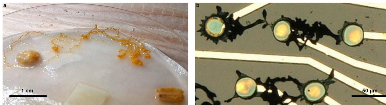
**Fig. 1** Structural analogy between slime mold and conducting polymer dendrites in water | (a) *Physarum polycephalum* growing in a Petri dish between oat flakes in water. (b) PEDOT:PSS growing on parylene C between voltage-supplied electrodes in water.
