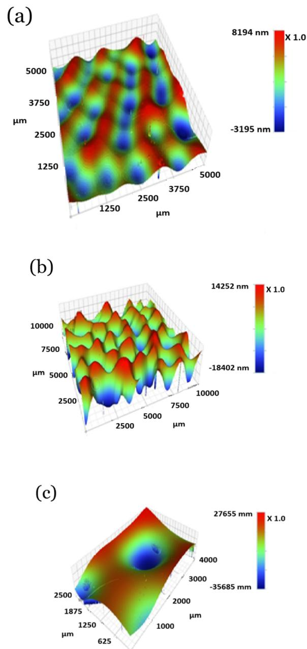
**Fig. 3** Optical profilometer 3D surface topography of PMMA thin films showing different honeycomb patterns drop casted using (a) 1 wt% PMMA at 30% relative humidity, (b) 5 wt% PMMA at 30% relative humidity, (c) 10 wt% PMMA at 30% relative humidity.
