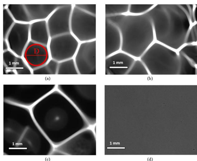
**Fig. 1** Optical micrograph of PMMA thin films casted under 30% relative humidity using an acetic acid solution with (a) 1 wt% showing an example of a honeycomb cell diameter ( $D$ ), (b) 5 wt% and (c) 10 wt% PMMA. (d) PMMA casted using 1 wt% PMMA solution under 20% relative humidity.
