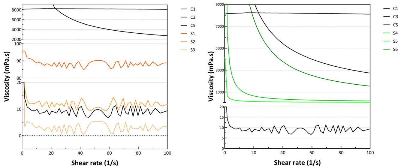
**Fig. 3** Rheological viscosity under increasing shear rate profiles of (left) sample resins with lower viscosity and (right) resins with higher viscosities were compared to respective control resins to establish shear-thinning nature and sufficient reduction of viscosity upon application of shear forces by the printers.
