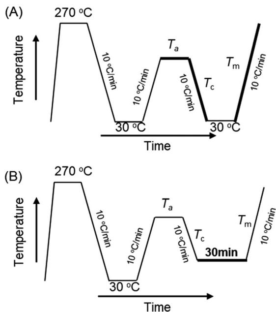
**Fig. 1** DSC temperature protocols for (A) nonisothermal and (B) isothermal crystallization after annealing at  $T_a$ .
