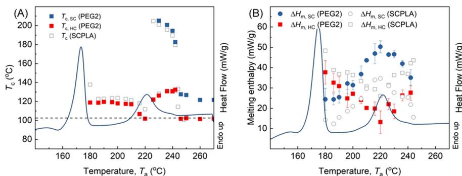
**Fig. 6** The  $T_a$  correspondence of (A)  $T_c$  and (B) melting enthalpies for plasticized SCPLA blend with 2 wt% PEG (labelled PEG2) as compared to neat SCPLA (labelled SCPLA). The error bars are not presented because of low measurement deviation.
