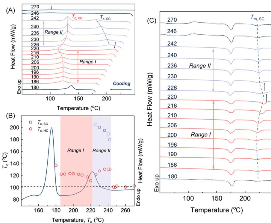
**Fig. 3** (A) DSC curves of SCPLA during cooling from different  $T_a$  to 30 °C at 10 °C min<sup>-1</sup>. (B) Corresponding  $T_{c,HC}$  and  $T_{c,SC}$  obtained from the DSC cooling curves. (C) Corresponding DSC heating curves from 30 °C to 270 °C at 10 °C min<sup>-1</sup> after the cooling from different  $T_a$ .
