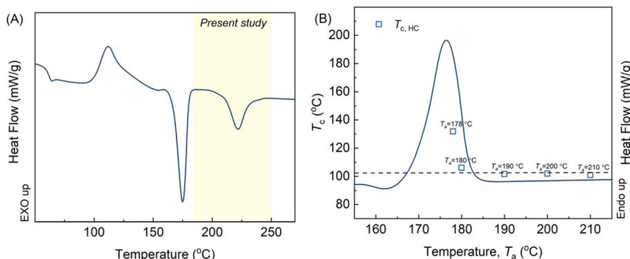
**Fig. 2** (A) DSC heating curve of SCPLA after cooling from 270 °C at 10 °C min<sup>-1</sup>. The thermal history of the samples was first removed at 270 °C for 3 min. (B) Endothermic peak of HC-crystal melting for HCPLA and the crystallization peak temperatures ( $T_{c,HC}$ ) during HCPLA cooling from different  $T_a$  (as x-axis).
