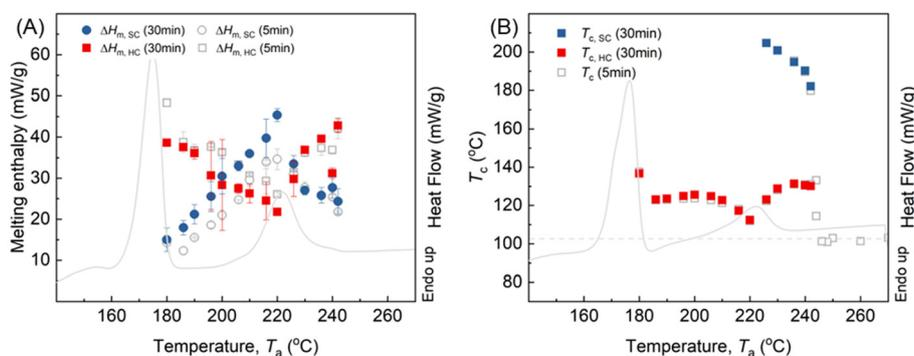
Fig. 4 (A) Melting enthalpies of HC ( $\Delta H_{m,HC}$ ) and SC-crystals ( $\Delta H_{m,SC}$ ) of SCPLA obtained upon cooling from different  $T_a$  for 5 min (empty symbols) or 30 min (solid symbols). (B) The corresponding  $T_c$  values of HC and SC-crystallization of SCPLA during cooling from different  $T_a$  for 5 min (empty symbols) or 30 min (solid symbols).
