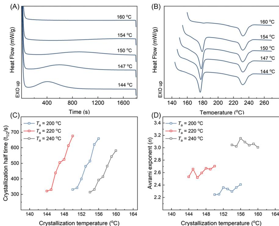
**Fig. 5** DSC curves of SCPLA (A) during isothermal crystallization at different temperatures after annealing at  $T_a = 220$  °C and (B) subsequent heating curves. (C) Crystallization half-time and (D) Avrami exponent of SCPLA isothermal crystallization at different temperatures after annealing at different  $T_a$  as denoted.
