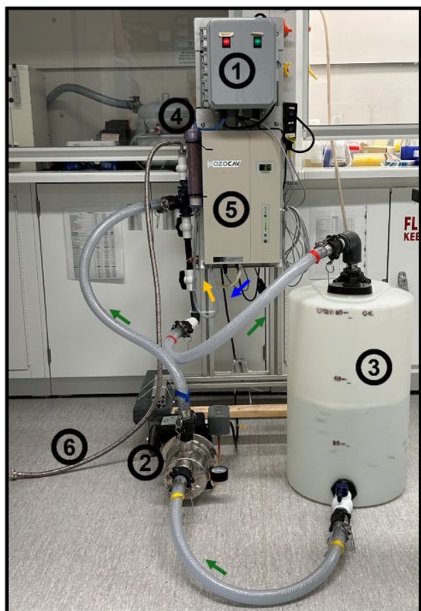
Figure 3 The closed-loop ozone micro/nanobubble generation setup developed by Econse Water Purification Inc. The system integrates a jet pump, desiccant column, corona discharge-based ozone generator, and cavitation unit to produce and circulate ozonized water enriched with entrained micro/nanobubbles. An outlet port allows sample collection during continuous recirculation.
