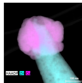
Fig. 4 High-resolution STEM-EDS micrograph of the tip of a ZnO rod (blue) with copper and copper oxide grown on the tip (purple).
