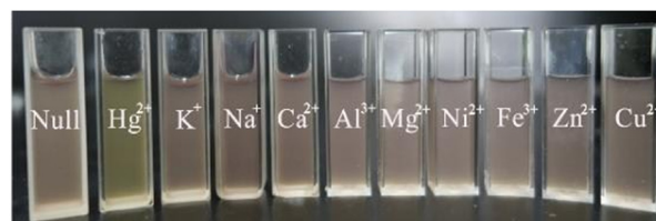
Fig. 9 The colorimetric change of PCN-224 in the presence of other metallic cations (5 \mu\text{M} ) and \text{Hg}^{2+} (5 \mu\text{M} ). Reproduced from ref. 89, with permission from the Royal Society of Chemistry, Yang et al. , RSC Adv. , 2016, 6 , 69807–69814, Copyright 2016.
