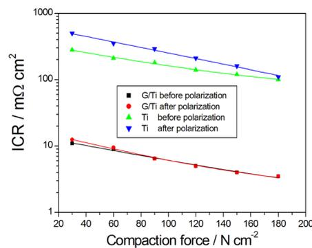
Fig. 11 ICR of untreated Ti and G/Ti before and after polarization. Reproduced from ref. 79, copyright 2019, with permission from Elsevier.
