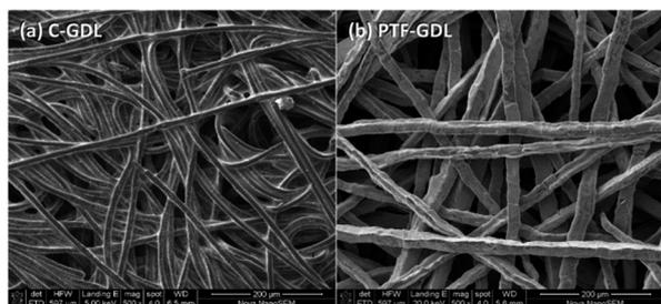
**Fig. 15** SEM images of (a) the C-GDL and (b) the PTF-GDL substrates. Reproduced from ref. 110, copyright 2023, with permission from Elsevier.
