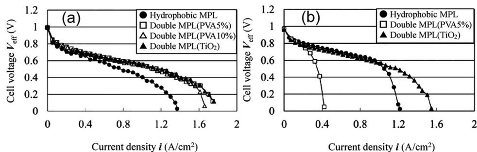
Fig. 16 (a) Influence of hydrophilic layer in double MPL-coated GDL (hydrophobic intermediate MPL: 20 mass% PTFE,  $d_m = 3 \mu\text{m}$ ,  $h_{\text{PTFE}} = 90 \mu\text{m}$ ) on PEMFC performance under (a) low humidity (anode: 60% RH, cathode: 0% RH) and (b) high humidity (anode: 100% RH, cathode: 100% RH). Reproduced from ref. 121, copyright 2013, with permission from Elsevier.
