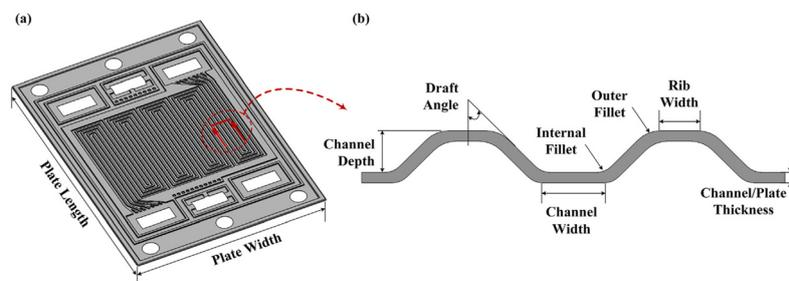
Fig. 2 Schematic diagram of a typical metallic BP: (a) overall; (b) cross section of the channels. Reproduced from ref. 9, copyright 2021, with permission from Elsevier.
