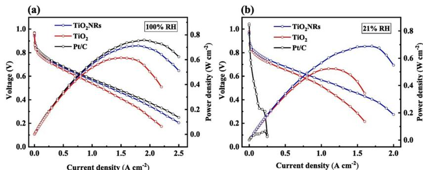
Fig. 17 Polarization and power density curves of PEMFCs with GDL-Pt/C, GDL-TiO<sub>2</sub> and GDL-TiO<sub>2</sub>NRs as anode at 60 °C and (a) 100% RH, (b) 21% RH. Reproduced from ref. 124, copyright 2024, with permission from Elsevier.
