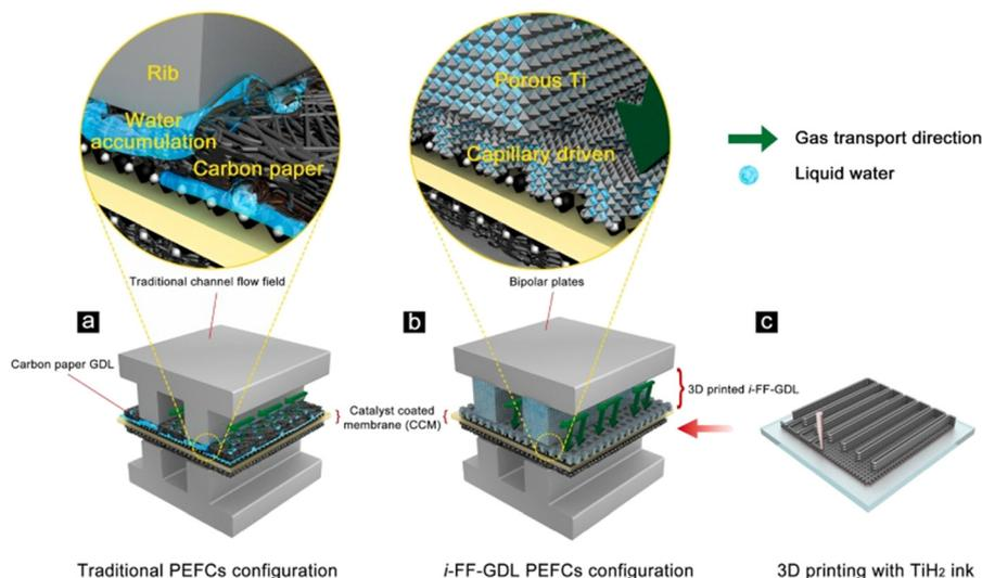
**Fig. 14** Schematic diagram of traditional PEMFC configuration (a), *i*-FF-GDL PEMFC configuration (b) and the 3D printing process (c). Reproduced from ref. 115, copyright 2021, with permission from Elsevier.
