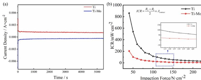
**Fig. 13** (a) Potentiodynamic polarization curves of Ti and Ti-0.35Mo. (b) ICR values after potentiostatic polarization for Ti and Ti-0.35Mo alloy. Reproduced from ref. 96, copyright 2024, with permission from Elsevier.
