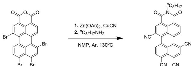
Fig. 1 Synthesis of CN<sub>4</sub>PMI.
