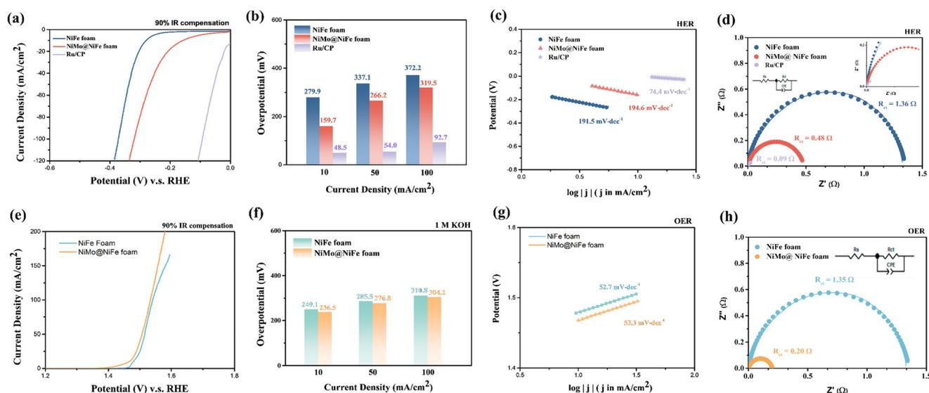
Fig. 4 Electrochemical performance of the NiFe foam, NiMo@NiFe foam, and Ru/CP electrodes for (a–d) the HER and (e–h) OER performance of the NiFe foam and NiMo@NiFe foam. (a and e) *iR*-compensated LSV curves, (b and f) overpotentials at 10, 50, and 100 mA cm<sup>-2</sup>, (c and g) Tafel slopes, and (d and h) Nyquist plots obtained from EIS measurements.
