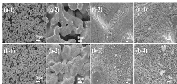
**Fig. 2** SEM images of (a-1)–(a-4): NiFe foam at magnifications of 100×, 1000×, 5000×, and 10 000×, respectively; (b-1)–(b-4): NiMo@NiFe foam at magnifications of 100×, 1000×, 5000×, and 10 000×, respectively.
