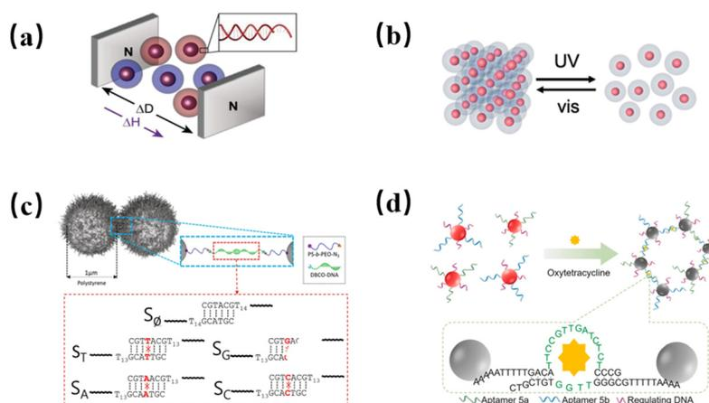
Fig. 4 Assembly of isotropic nanoparticles. (a) Assembly of nanoparticles in magnetic fields.<sup>68</sup> Copyright 2019, John Wiley and Sons. (b) Disconnection under ultraviolet light.<sup>70</sup> Copyright 2020, John Wiley and Sons. (c) Mismatch of some bases.<sup>72</sup> Copyright 2024, American Chemical Society. (d) Split adaptor-guided assembly.<sup>80</sup> Copyright 2025, Elsevier.
