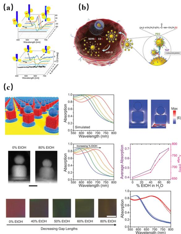
**Fig. 9** (a) CD spectra of gold nanoparticle helical structures.<sup>22</sup> Copyright 2022, American Chemical Society. (b) Schematic representation of Y-DNA-driven construction of Au NP chiral C<sub>30</sub>S<sub>5</sub>S<sub>10</sub> NSs with enhanced CD and SERS signals. Copyright 2020, John Wiley and Sons. (c) Reconfigurable optical properties. Scale bar, 50 nm.<sup>19</sup> Copyright 2018, AAAS.
