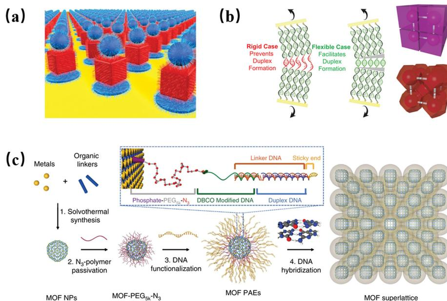
**Fig. 5** Assembly of anisotropic nanoparticles. (a) Each unit cell of the NP superlattice consists of a gold surface, circular disk, and cube.<sup>19</sup> Copyright 2018, AAAS. (b) Rigid DNA strands and flexible DNA strands.<sup>81</sup> Copyright 2024, AAAS. (c) Crystallization engineering of MOF particles.<sup>18</sup> Copyright 2020, Springer Nature.
