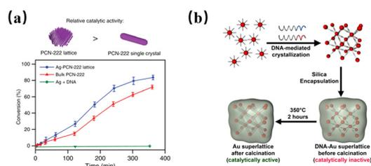
**Fig. 8** (a) The photocatalytic activity of the 2D PCN-222 nanorod superlattices is examined.<sup>18</sup> Copyright 2020, Springer Nature. (b) Synthesis of catalytically active DNA-nanoparticle superlattices.<sup>116</sup> Copyright 2015, American Chemical Society.
