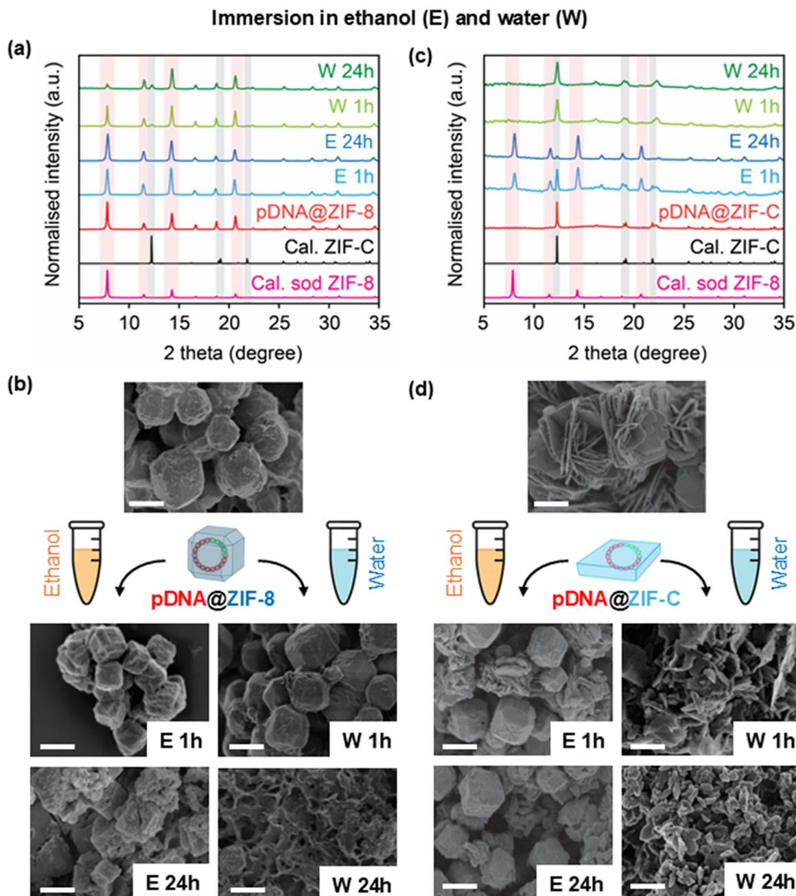
Fig. 5 Stability assessment of pDNA@ZIF-8 (a and b) and pDNA@ZIF-C (c and d) after incubation in ethanol (EtOH, E) and water (H<sub>2</sub>O, W). The powder material incubated at different times was collected and analyzed via (a and c) XRD and (b and d) SEM. Scale bar: 500 nm.
