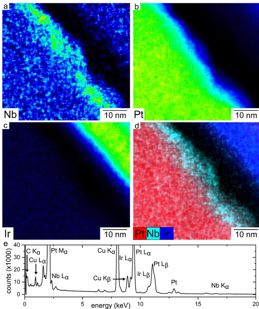
**Fig. 3** (a–c) Individual and (d) overlapping elemental maps for the (a) Nb K $\alpha$ , (b) Pt L $\alpha$ , and (c) Ir signals as obtained by energy dispersive X-ray spectroscopy (EDS) measurements of a cross-section obtained from a Nb<sub>2</sub>O<sub>5</sub> coated polycrystalline Pt substrate. (e) A representative spectrum obtained using EDS techniques with labelled transitions.
