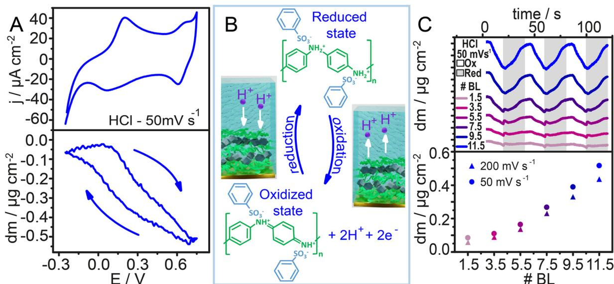
Fig. 5 (A) Cyclic voltammetry and QCM mass change curves for the assembly in 0.1 M HCl at 50  $\text{mV s}^{-1}$ . (B) Ionic exchange from the LbL assembly during the redox reaction. (C) Mass change as a function of time during the redox reaction for films of different number of deposition cycles (above). Mass exchange value for the different stages in the assembly process (below).
