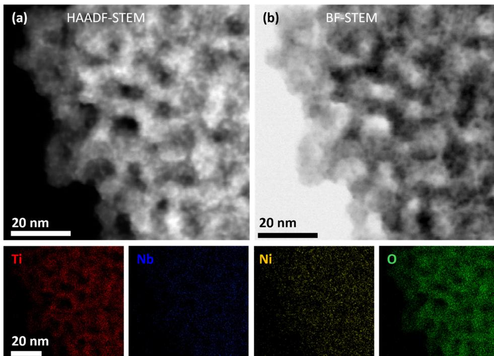
Fig. 3 (a) HAADF-STEM, (b) BF-STEM, and corresponding EDX mapping images for  $50\text{NiO-Nb}_x\text{Ti}_{1-x}\text{O}_2$  thin films are shown in the bottom panel. The corresponding EDX spectra are shown in Fig. S3.
