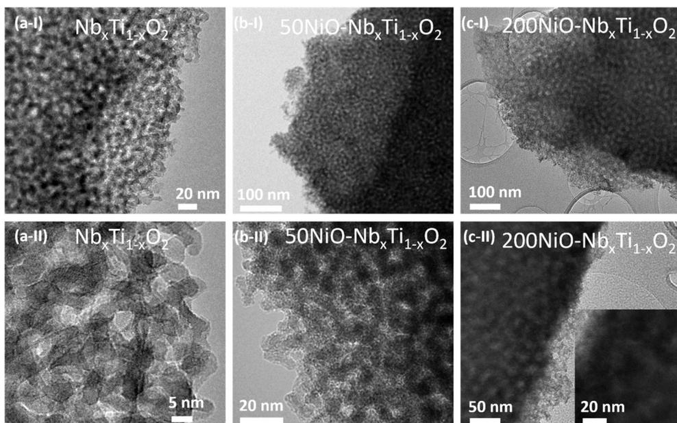
Fig. 2 BF-HRTEM images of (aI and II)  $\text{Nb}_x\text{Ti}_{1-x}\text{O}_2$ , (bI and II)  $50\text{NiO-Nb}_x\text{Ti}_{1-x}\text{O}_2$ , and (cI and II)  $200\text{NiO-Nb}_x\text{Ti}_{1-x}\text{O}_2$  nanostructures.
