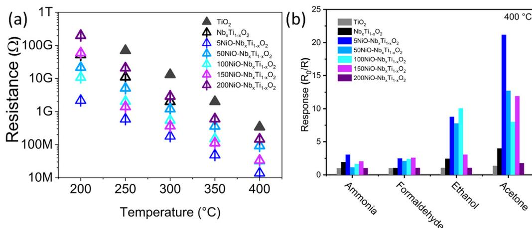
Fig. 4 (a) Electrical resistance of  $\text{Nb}_x\text{Ti}_{1-x}\text{O}_2$  and  $\text{NiO-Nb}_x\text{Ti}_{1-x}\text{O}_2$  heterostructures in dry air at a temperature range of 200–400 °C. (b) Chemoresistive sensing response of  $\text{Nb}_x\text{Ti}_{1-x}\text{O}_2$  and  $\text{NiO-Nb}_x\text{Ti}_{1-x}\text{O}_2$  nanostructures to various gases (40 ppm) including ammonia, formaldehyde, ethanol and acetone at 400 °C.
