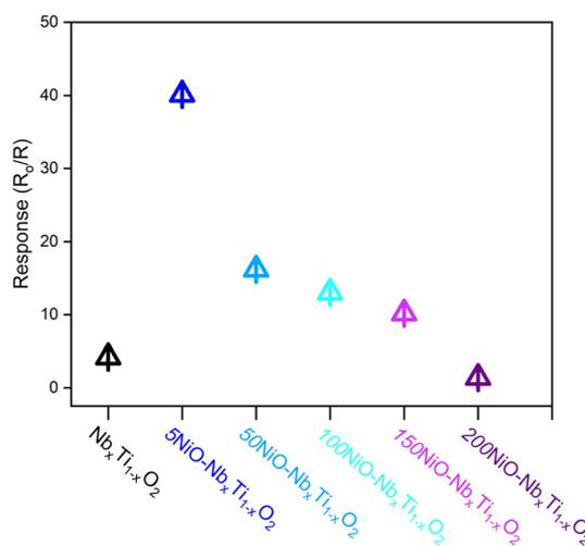
Fig. 7 Chemoresistive response of the 5NiO–Nb<sub>x</sub>Ti<sub>1-x</sub>O<sub>2</sub> thin films as a function of the NiO layer thickness toward 40 ppm of acetone at 300 °C.
