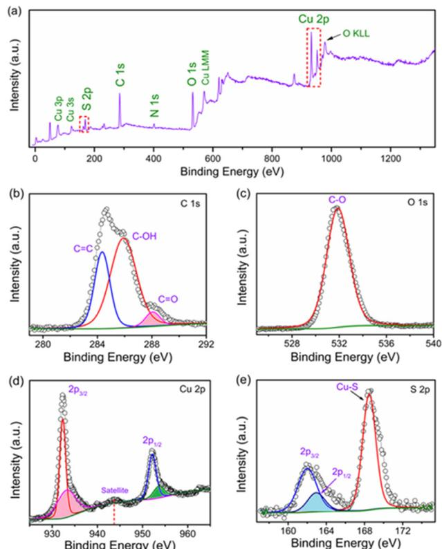
Fig. 2 (a) XPS full scan survey spectrum of the copper sulfide thin film. High resolution spectra of the (b) C 1s, (c) O 1s, (d) Cu 2p, and (e) S 2p regions.
