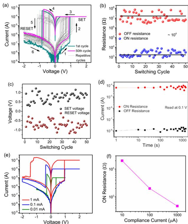
**Fig. 3** (a)  $I$ - $V$  characteristics of the Cu/Cu<sub>2-x</sub>S/ITO memristive device showing bipolar digital RS behavior, (b) ON and OFF state resistances plotted as function of switching cycles, (c) plot of SET and RESET voltage with switching cycles, (d) retention test of the ON and OFF state, (e) multilevel  $I$ - $V$  characteristics observed in the memristive device with varying compliance current, and (f) plot of ON state resistance ( $R_{ON}$ ) with compliance current (CC).
