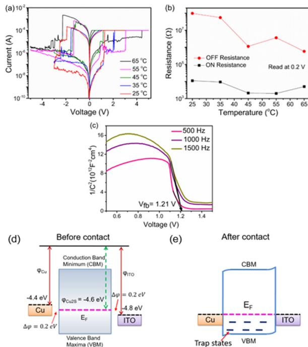
**Fig. 6** (a)  $I$ - $V$  characteristics of the first sweep cycle with temperature ranging from 25 to 65 °C, (b) ON and OFF resistance plots with temperature, and (c) Mott-Schottky plots of  $\text{Cu}_{2-x}\text{S}$ . Schematic of the energy band diagram of the  $\text{Cu}/\text{Cu}_{2-x}\text{S}/\text{ITO}$  memristive device (d) before and (e) after contact.
