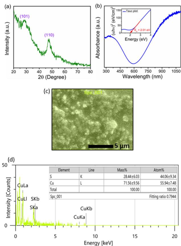
**Fig. 1** (a) XRD pattern of the CBD copper sulfide film onto the ITO/PET substrate. (b) UV-visible absorption spectra of CBD copper sulfide film. The inset of (b) shows the determination of the band gap energy from the Tauc plot. (c) SEM image and (d) EDS spectra of copper sulfide thin film.
