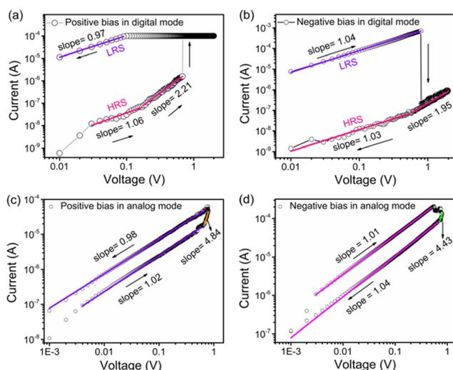
**Fig. 5** log-log plots of a digital  $I$ - $V$  curve for the (a) SET process and (b) RESET process in the  $\text{Cu}/\text{Cu}_{2-x}\text{S}/\text{ITO}$  memristive device. log-log plots of an analog  $I$ - $V$  for the first (c) positive and (d) negative voltage sweep of the device.
