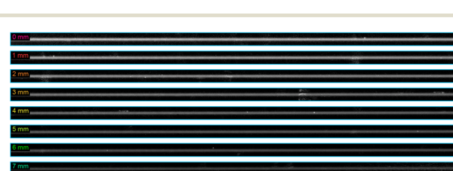
Fig. 4 Examples of microscopic images showing side-scattered light from a water-filled silica capillary with an inner channel diameter of d_c = 17.8 \mu\text{m} ( \lambda_0 = 532 \text{ nm} ). Each image represents a 1.41 mm-long section along the capillary. The eight images are vertically stacked, with the total distance from the capillary entrance indicated by the labels on the left.
