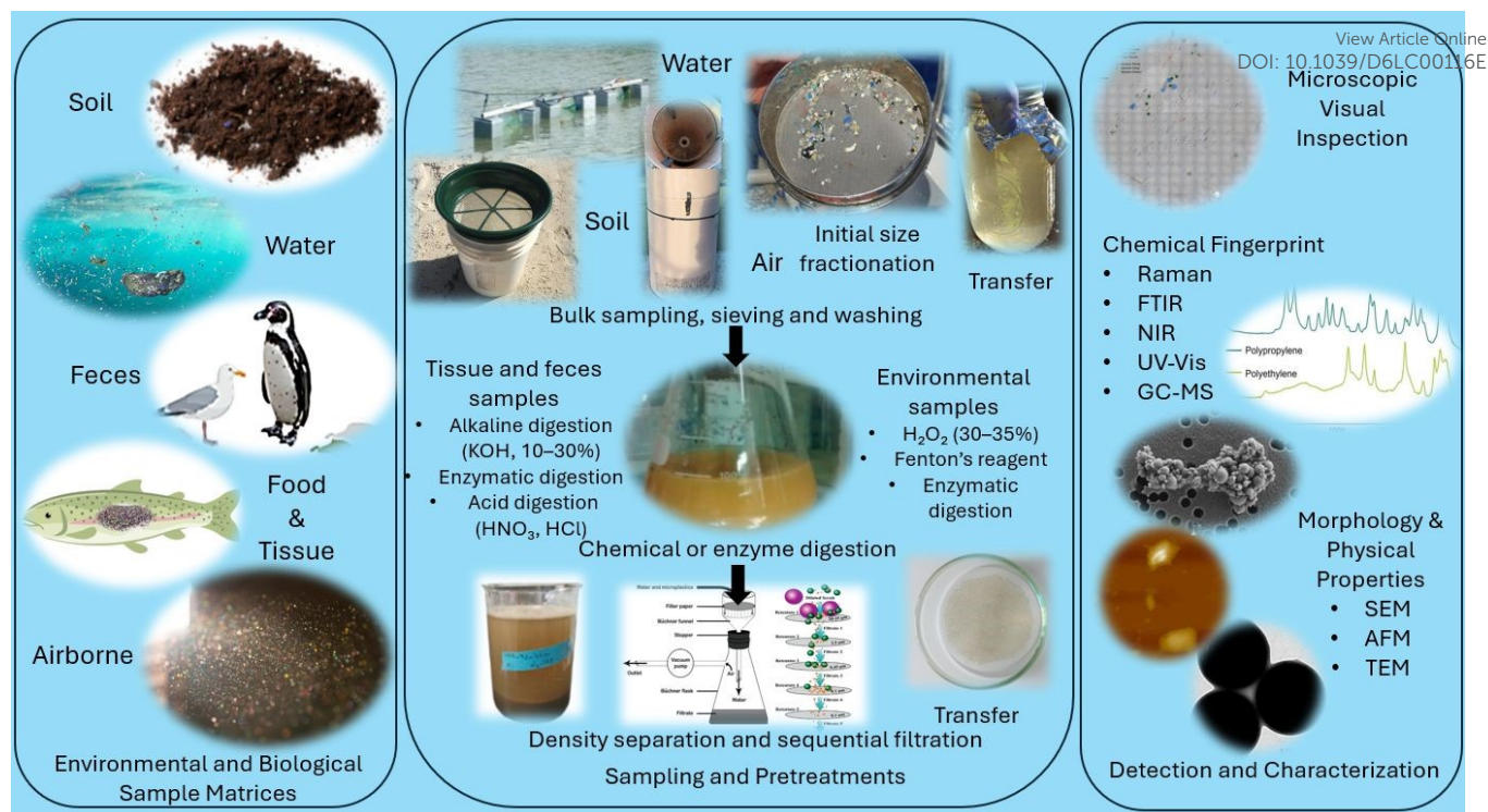
Fig. 1 Conventional workflow of MPs/NPs sampling, detection, and characterization. In general, initial sampling step relies on bulk sampling, followed by size-based fractionation and collection into glass container transferred back to laboratory for further processing. Then, different types of samples utilize different digestion reagents followed by density based separation, the supernatant goes through sequential filtration and isolate particles of interests of variety of sizes, finally trapped on membrane filters for characterizations. Depends on the nature of downstream characterization techniques, further processing of the filter paper is required.
