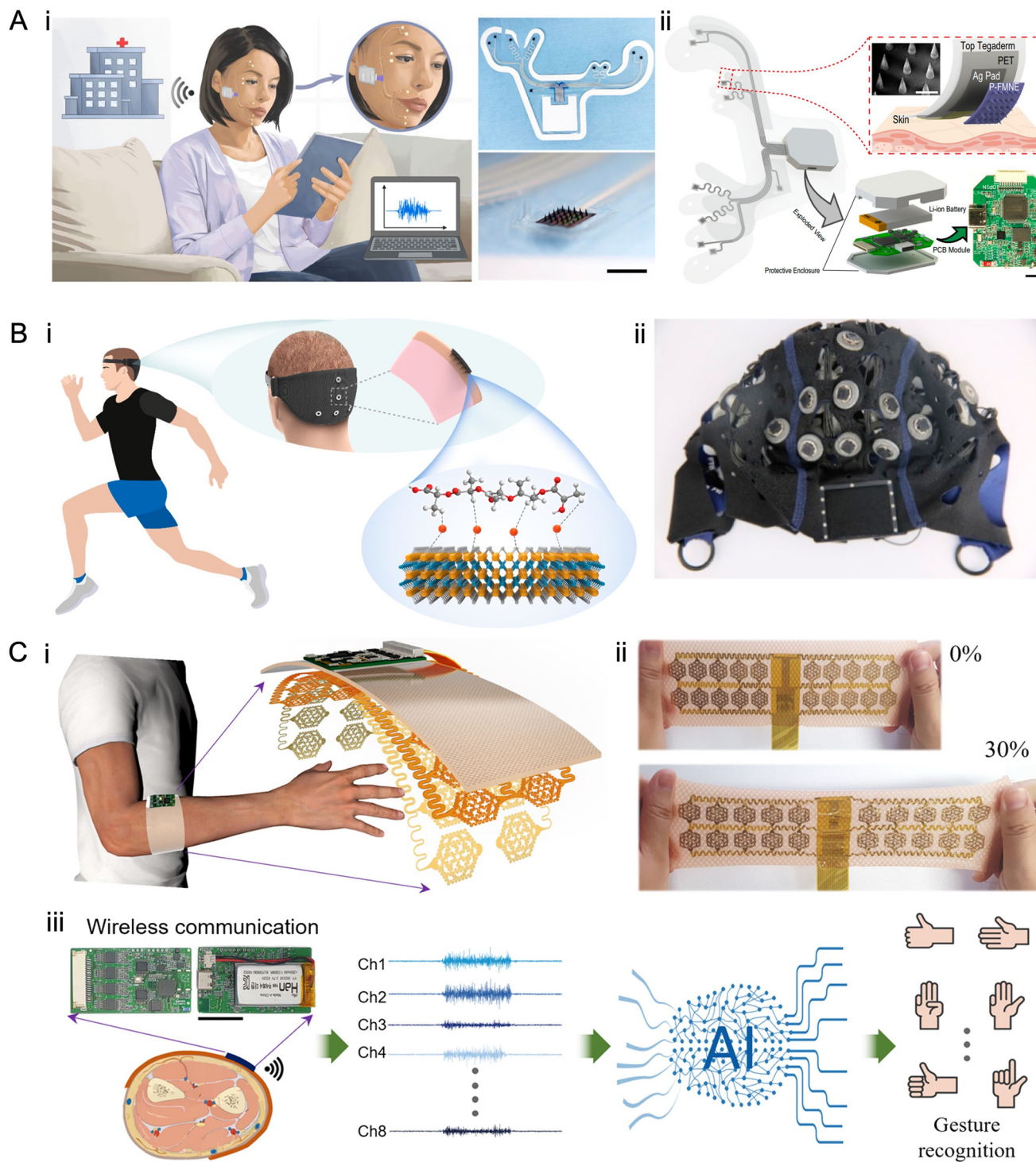
Fig. 9 MN wearable devices for electrophysiological signal monitoring. (A) Integration of MN electrodes with flexible electronics for facial biosensing: (i) illustration of a soft wearable electronic mask for facial EMG monitoring; (ii) design of the electrode component and PCB module. Reproduced from ref. 122 under the CC-BY 4.0 license. (B) Integration of MN electrodes as brain-computer interfaces with an EEG scalp cap: (i) Mxene MN electrode as a brain-computer interface; (ii) the wearable EEG cap. Reproduced with permission from ref. 117. Copyright 2025, American Chemical Society. (C) Integration of MN electrode devices with artificial neural networks for enhanced bioelectrical signal interpretation: (i) wearable EMG sensor for real-time monitoring of EMG signals; (ii) original and stretched wearable EMG sensor; (iii) gesture recognition by a graph neural network using transmitted data from the EMG sensor. Reproduced from ref. 126 under the CC-BY 4.0 license.
