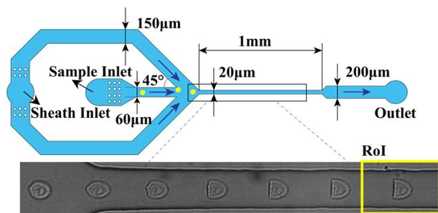
**Fig. 8** Schematic diagram of the microchannel geometry. The photo inset illustrates the transient deformation of a cell. The yellow box represents the region of interest (RoI) for image acquisition where the cell has reached steady deformation.
