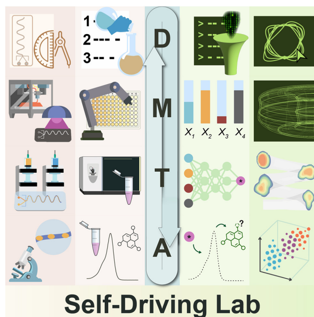
Fig. 1 Self-driving lab workflow. Physical laboratory components (left) are integrated with digital tools (right) to create a streamlined design–make–test–analyze (DMTA) cycle. Central arrow illustrates the iterative DMTA process flow. Each column demonstrates different aspects of automated experimentation in both physical and digital settings: reactor/process design (outer), and material/molecular design (inner), enabling autonomous scientific discovery through continuous optimization loops.
