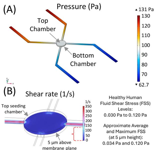
**Fig. 3** CFD simulations of the CoCM microfluidic chip design. (A) Simulated pressure drop across the passive microfluidic device when inlet reservoirs are initially filled. (B) Shear rate distribution within the whole seeding chamber, showing an FSS slide at a height of 5  $\mu\text{m}$  above the membrane, where the cells are adhered. The analysis ensures that cells are exposed to physiologically relevant FSS levels<sup>42</sup> that support cell viability for human kidney cells.
