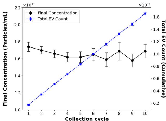
Fig. 6 Punctuated operation of the electrophoretic enrichment device. EV samples were sequentially processed in 100  $\mu\text{L}$  aliquots ( $Q = 10 \mu\text{L min}^{-1}$ ,  $t = 10 \text{ min per cycle}$ ) across 10 consecutive collection cycles.
