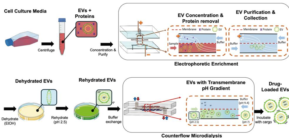
**Fig. 1** Microfluidic-enabled workflow employing an electrophoretic enrichment chip enabling concentration and purification of EVs from cell culture media, and a counterflow microdialysis chip supporting transmembrane pH gradient generation to prepare EVs for drug loading.
