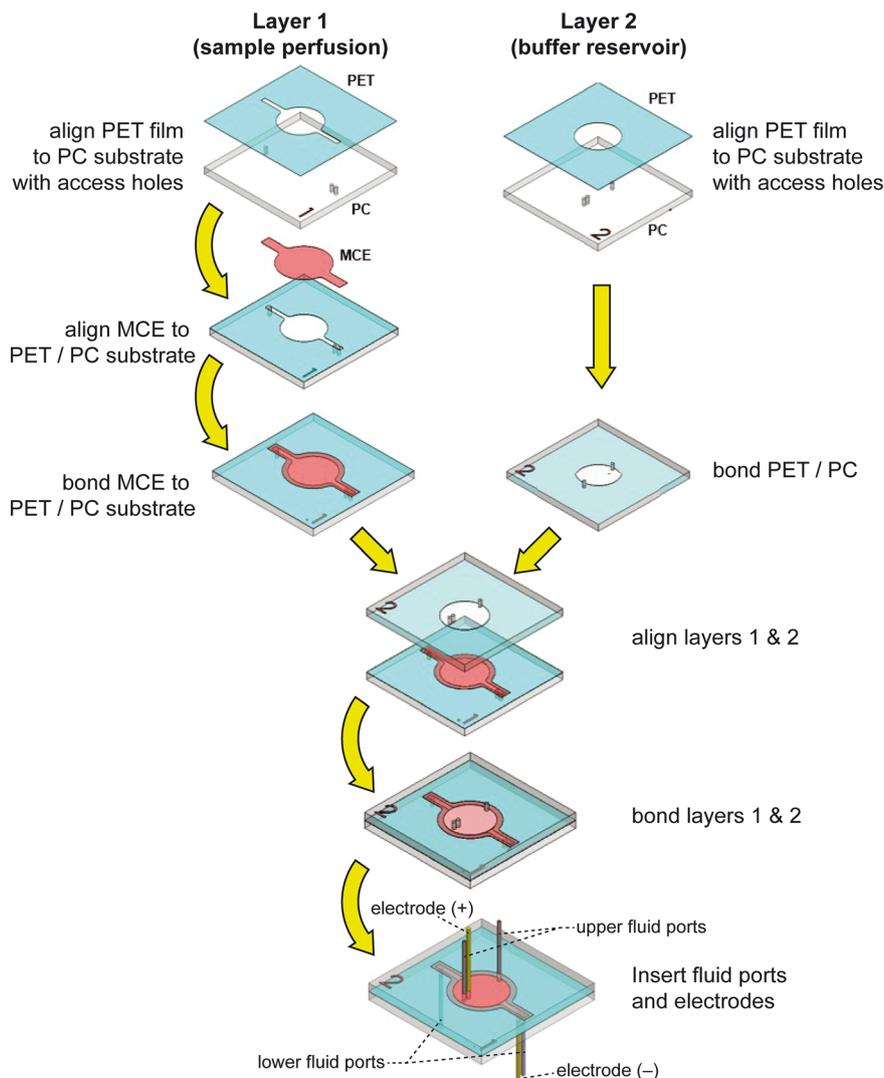
**Fig. 2** Fabrication process for the electrokinetic chips for EV concentration and purification. Adhesive PET tape layers are used to define the channel and reservoir geometry, and bonded with polycarbonate substrates containing pre-drilled holes for fluidic and electrical interfacing. A patterned MCE membrane is positioned between the mating PET/PC layers. Needle ports and electrodes are inserted into the PC layers after bonding.
