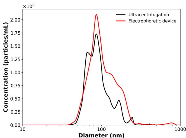
Fig. 4 Particle size distributions after enrichment by conventional ultracentrifugation, and after microfluidic electrophoretic enrichment at  $10 \mu\text{L min}^{-1}$  flow rate and 60 V bias for 10 min.
