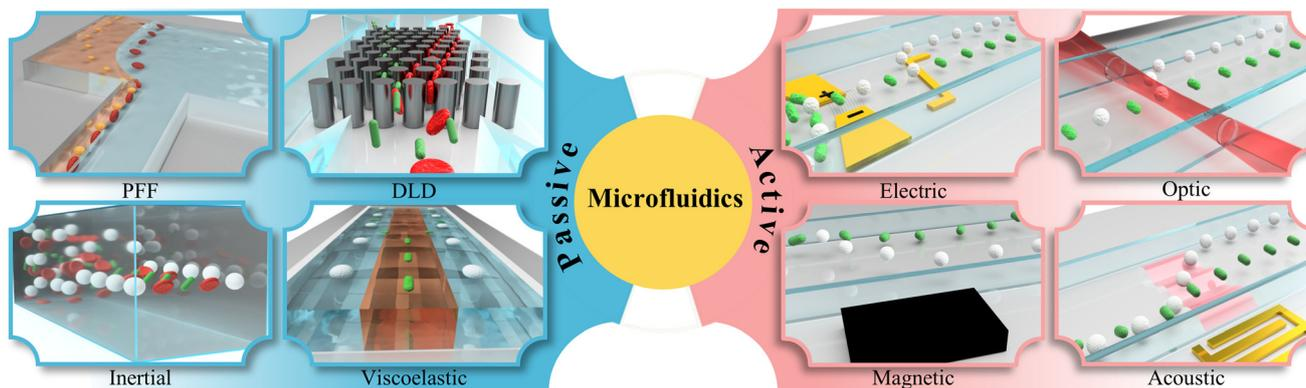
**Fig. 1** Schematic overview of microfluidic shape-based separation techniques categorized into passive and active methods. Passive techniques such as deterministic lateral displacement (DLD), inertial, viscoelastic, and pinched flow fractionation (PFF) utilize channel geometries and intrinsic fluid forces, while active techniques based on electric, optical, magnetic, and acoustic fields apply external forces for enhanced and tunable particle manipulation.
