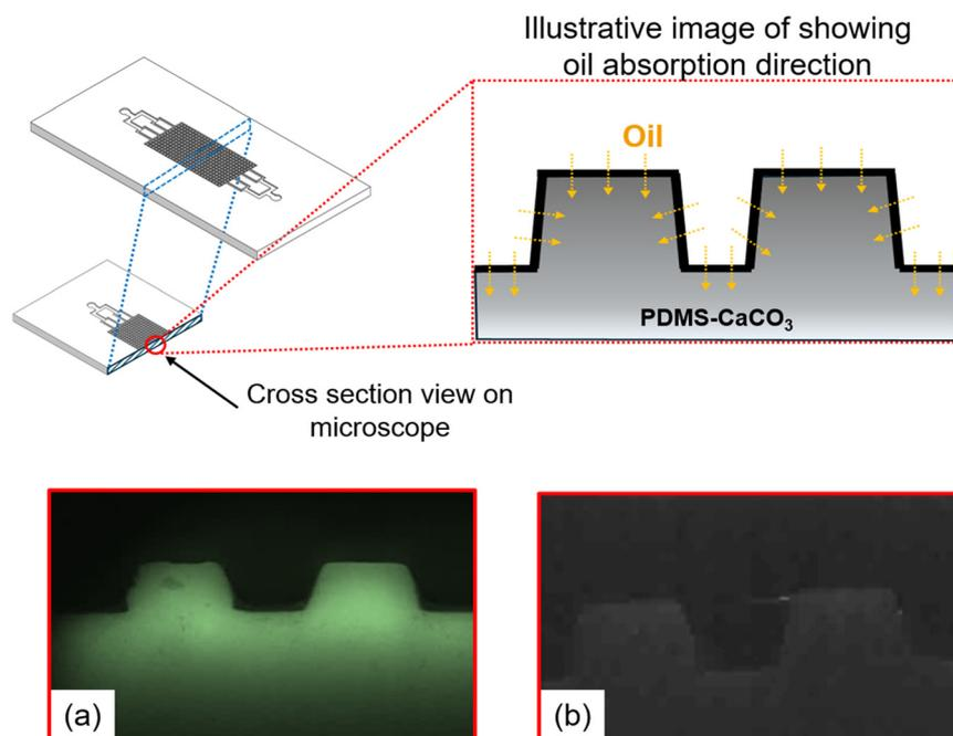
**Fig. 6** Schematic of the PDMS- $\text{CaCO}_3$  microchannel and fluorescence microscopy validation of oil absorption. The magnified cross-section highlights oil uptake (yellow arrows) into the micropillar walls and base. (a) Oil-exposed channel shows strong fluorescence, confirming oil absorption. (b) The control channel shows no fluorescence, indicating no oil presence; image brightness was enhanced for visibility due to low signal in the dark field.
