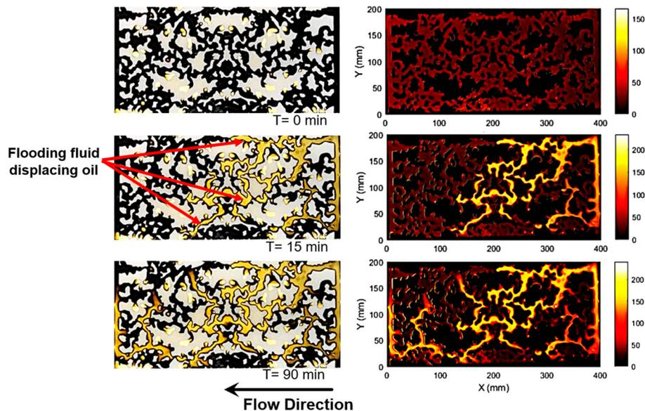
**Fig. 9** Flooding progression in a randomly structured microfluidic network. Left: experimental snapshots at different time points (dark region represents oil and light region represents flooding fluid). Right: MATLAB-processed images showing pixel intensity mapping used to visualize oil displacement.
