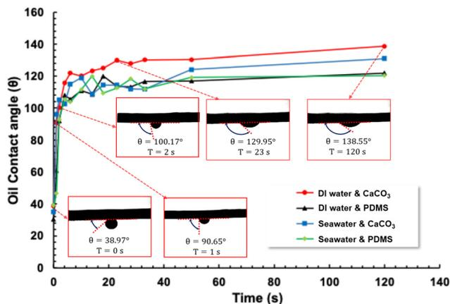
Fig. 5 Time-dependent oil contact angle measurements on PDMS– $\text{CaCO}_3$  and PDMS surfaces in DI water and seawater. The five experimental images show oil droplet profiles at different times (0 s, 1 s, 2 s, 23 s, and 120 s) on the PDMS– $\text{CaCO}_3$  surface immersed in DI water.
