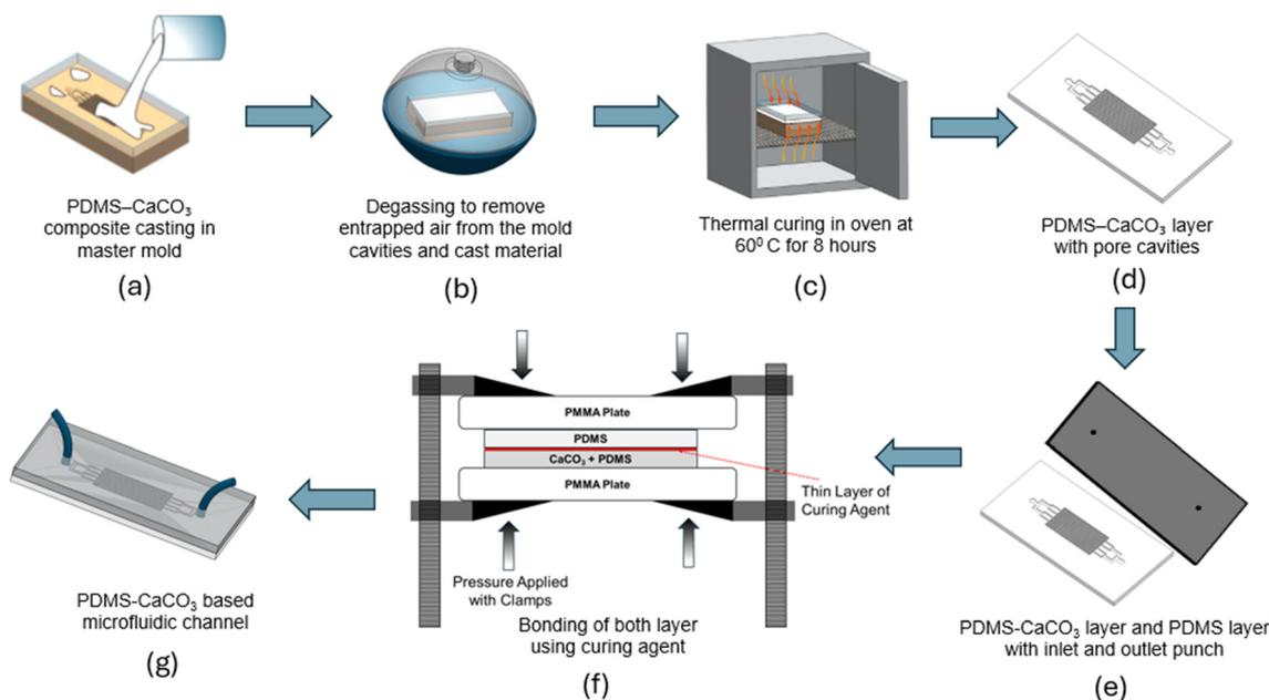
**Fig. 2** Fabrication procedure for the PDMS- $\text{CaCO}_3$  microfluidic device: (a) mold casting, (b) degassing, (c) curing, (d) trimming the bottom channel with pore cavity, (e) preparing the top PDMS layer, (f) bonding the PDMS- $\text{CaCO}_3$  and PDMS layers, and (g) connecting inlet and outlet tubing.
