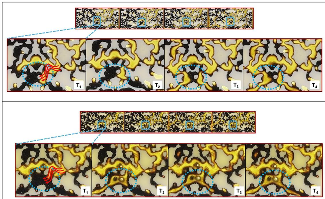
**Fig. 11** Image sequence showing oil displacement in the random porous network using seawater–concrete–CO<sub>2</sub> (top) and SDS (bottom) flooding. Each sequence captures four time points:  $T_1 = 8$  min,  $T_2 = 10$  min,  $T_3 = 15$  min, and  $T_4 = 30$  min. The blue dotted circles indicate the region of interest used to observe pore-scale displacement.
