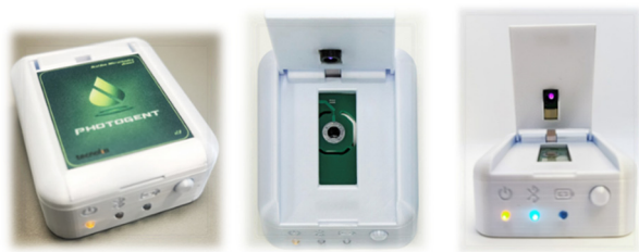
Fig. 6 External view of the portable colorimetric reader (A). Image of the measurement chamber, customized to fit the geometry of the microfluidic chip (B). Working device with purple emitting mode (C).
