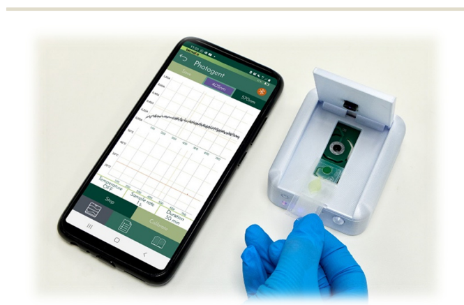
Fig. 2 Operation of the photogent reader. A user inserts the microfluidic chip into the reader while the smartphone app shows the real-time absorbance signal recorded during the enzymatic assay.
