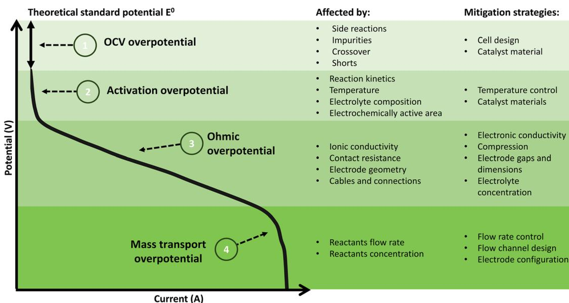
Fig. 2 Cell polarization curve with detailed overpotentials and mitigation strategies.
