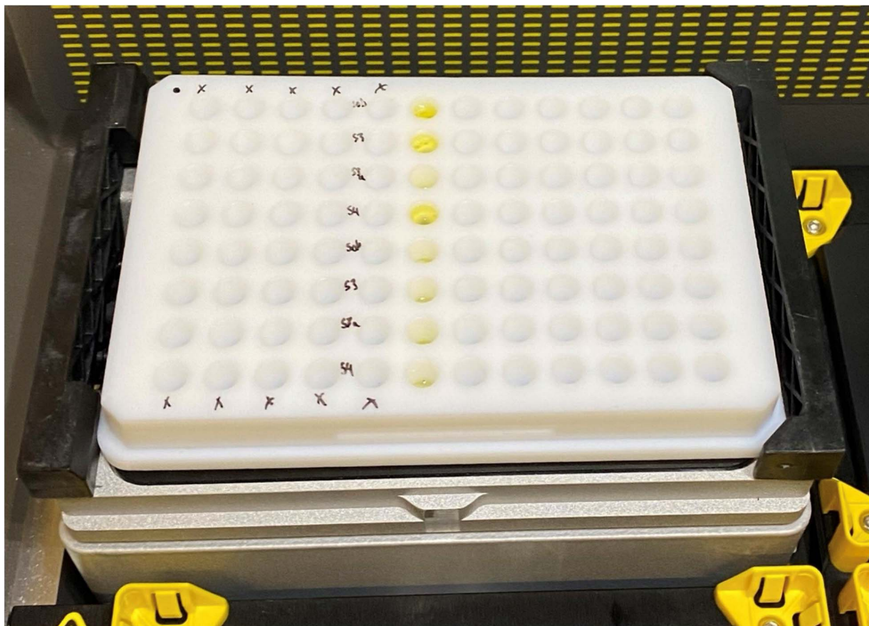
Fig. 2 Picture of the custom-machined PTFE 96-well plate on the heater/shaker during dissolution. The sixth column from the left was being used for dissolution, showing the yellow-colored acids reacting within the wells.
