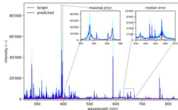
Fig. 8 Visualization of PDS approach, illustrating below-average to worst-case transfer quality and effectiveness. Spectra are transferred from Earth at 15 mJ laser energy to low-vacuum. The plot shows the mean transferred spectra alongside the target atmospheric spectra, with shaded regions indicating their respective standard deviations.
