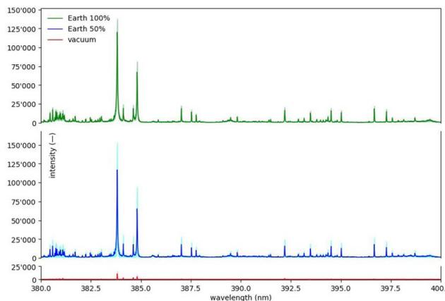
Fig. 3 Comparison of LIBS spectra for 380–400 nm spectral range, acquired under different conditions for the same sample. The solid line indicates the mean spectrum across repeated measurements for the respective condition, while the shaded region represents its standard deviation. The visualized sample is a synthetic lunar material rich in aluminum and aluminum oxide.
