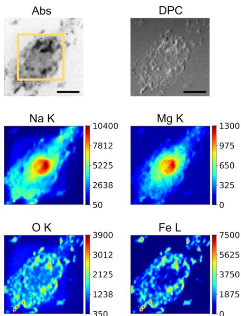
Fig. 4 XRF distribution maps of Na, Mg, O and Fe, shown together with the corresponding absorption (Abs) and differential phase contrast (DPC) STXM images of the GBM cell. The scale bar is  $10 \mu\text{m}$ . The yellow square indicates the area where the XANES stack was measured.
