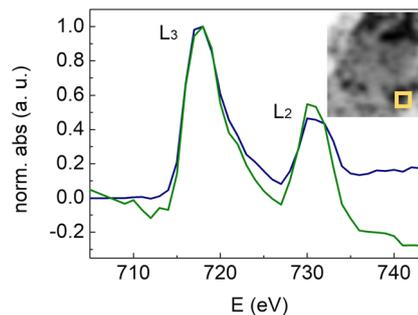
Fig. 5 Fe L-edges XANES spectra of a portion of the selected subarea of GBM cell exposed to Fe oxide NPs acquired in STXM (blue) and XRF (green) mode. The inset shows the attenuation in the  $14.5 \times 15.5 \mu\text{m}^2$  area at the incident energy of 726 eV. The yellow square of  $2 \times 2 \mu\text{m}^2$  indicates the portion of the area from which the spectrum was integrated.
