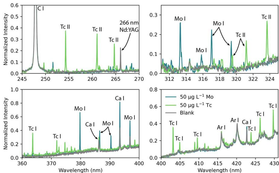
Fig. 1 Identified strong emissions for Tc in trace conditions. Spectra for a blank sample and nominally  $50 \mu\text{g mL}^{-1}$  Mo. Each subplot shows different wavelength windows from the same spectra.
