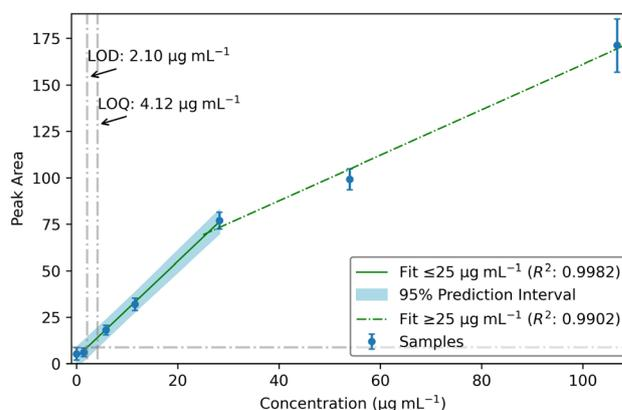
Fig. 5 Self-absorption behavior of the 323.70 nm Tc II emission peak collected on the CZ ICCD spectrometer versus concentration. Note that error bars correspond to  $2 \times$  standard error ( $n = 60$ ).
