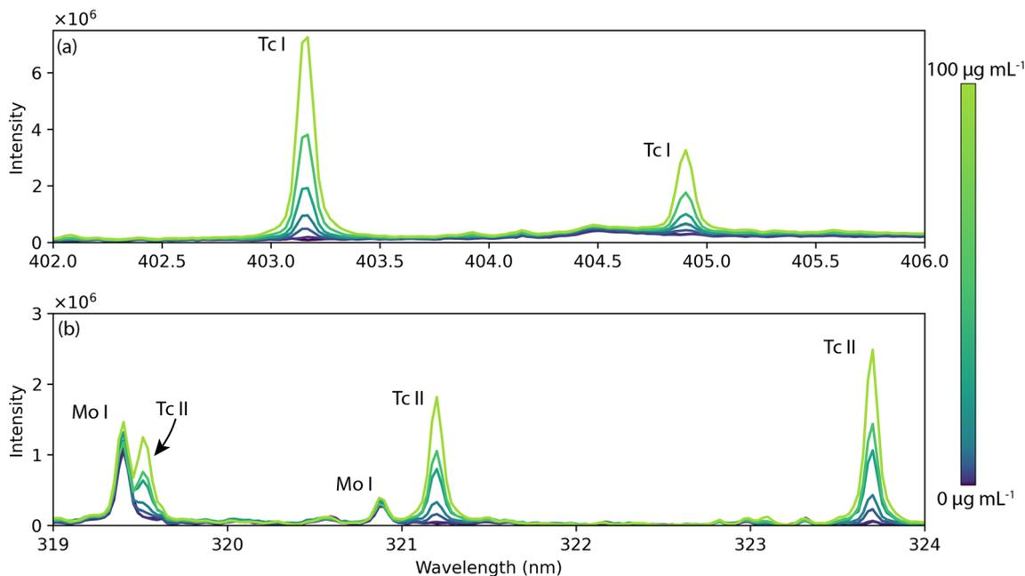
Fig. 3 LIBS spectra as a function of Tc concentration collected on the CZ ICCD spectrometer. Two spectral windows were selected because of their (a) strong neutral emissions and (b) weak ionized emissions with Mo interferences.
