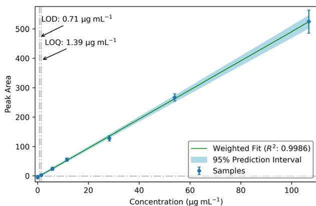
Fig. 4 Tc I 403.16 nm emission signal from LIBS collected using the CZ ICCD spectrometer as a function of Tc concentration. The error bars correspond to  $2 \times$  standard error ( $n = 60$ ).
