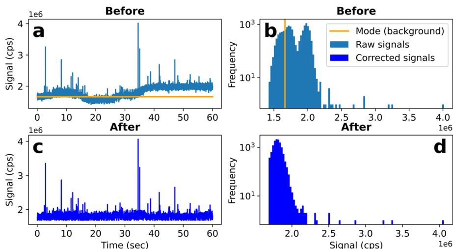
**Fig. 1** Baseline-drift correction *via* Sparta for <sup>197</sup>Au<sup>+</sup> (10 ppb, ionic standard in ultrapure water, 5 ms dwell time). (a) Raw signals (signal vs. time) before correction. (b) Raw histograms (frequency vs. signal) before correction. (c) Corrected signals (signal vs. time). (d) Corrected histograms (frequency vs. signal).
