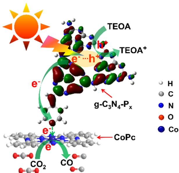
**Scheme 1** Charge transfer diagram for CO<sub>2</sub> photoreduction over CoPc/g-C<sub>3</sub>N<sub>4</sub>-P<sub>x</sub> hybrid photocatalysts under visible-light illumination.
