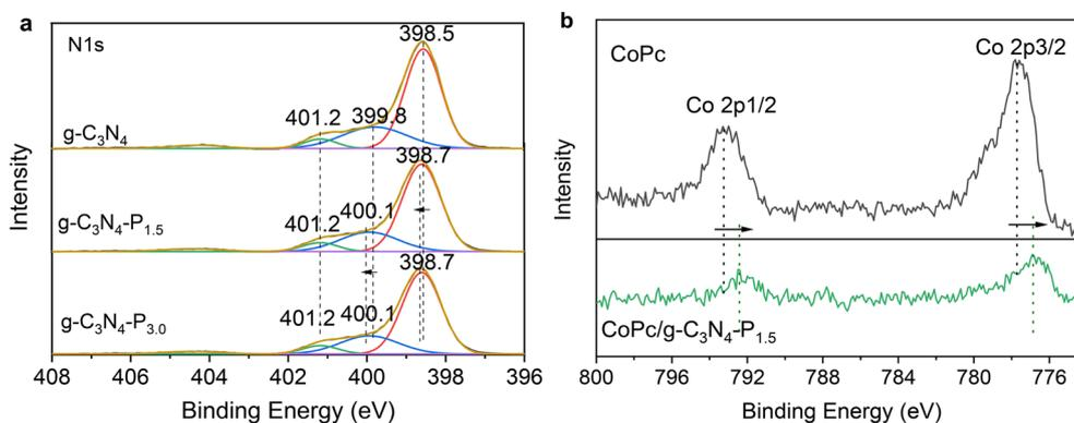
Fig. 3 High-resolution XPS spectra of (a) N 1s of the  $g\text{-C}_3\text{N}_4$ ,  $g\text{-C}_3\text{N}_4\text{-P}_{1.5}$ , and  $g\text{-C}_3\text{N}_4\text{-P}_{3.0}$  samples, and (b) Co 2p of CoPc and the CoPc/ $g\text{-C}_3\text{N}_4\text{-P}_{1.5}$  hybrid catalyst.
