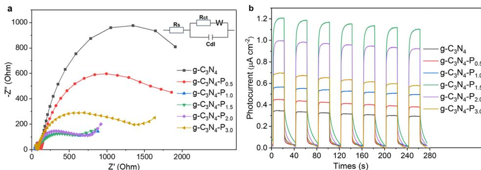
Fig. 5 (a) EIS Nyquist plots (the inset shows the equivalent circuit), and (b) the transient photocurrent response ( $I-t$ ) of the pristine  $g\text{-C}_3\text{N}_4$  and  $g\text{-C}_3\text{N}_4\text{-P}_x$  ( $x = 0.5-3.0$ ) samples.
