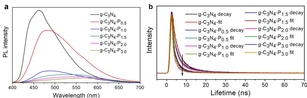
Fig. 6 (a) Steady-PL and (b) TR-PL kinetics decay spectra probed at 460 nm for the pristine  $g\text{-C}_3\text{N}_4$  and as-synthesized  $g\text{-C}_3\text{N}_4\text{-P}_x$  ( $x = 0.5-3.0$ ) samples at 370 nm excitation.
