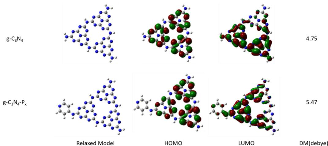
**Fig. 7** Optimized structures, calculated dipole moments, and isodensity surface plots of the HOMO and LUMO for g-C<sub>3</sub>N<sub>4</sub> and g-C<sub>3</sub>N<sub>4</sub>-P<sub>x</sub> model structures.
